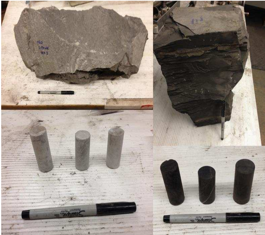
Figure 2.7. Images of D Chalk (left) and D Marl (right) samples. The D chalk is a clean chalk while the D marl contains clay, pyrite, and organic matter.
