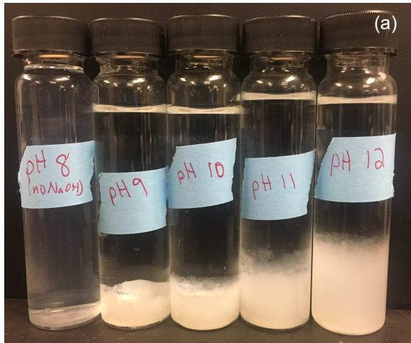
Figure 3-8. MD concentrate of 8x MU-S UFP at pH 8 and adjusted to pH 9-12 (left) (b) Concentrations of ions in the supernatant and the floc of the MD concentrate 8x MU-S UFP after 87% recovery.
