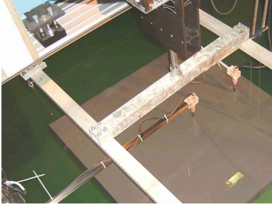
Figure 5.13: The experimental configuration: the PVC slab is suspended in water by cables attached to its corners. The source hydrophone remains in a fixed position while a robotic arm controls the position of the receiver hydrophone.
