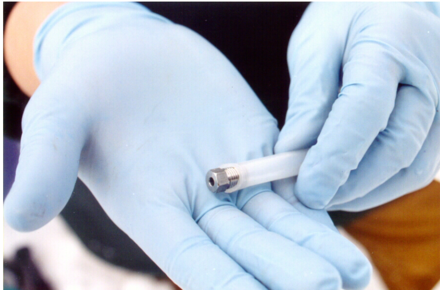
Figure 5-1: The Waterra pumping system utilized for groundwater removal
