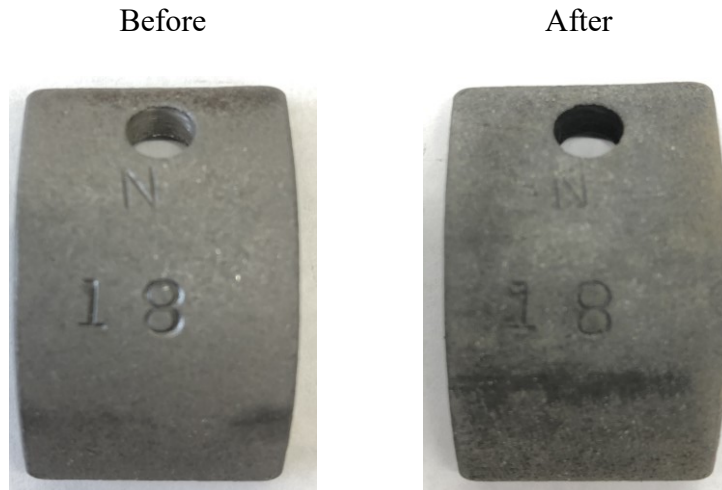
Figure 5.19 Tested steel coupon before and after soaking it at 300°F and 1,000 psi using 14 wt% LA:GA acid mixture solution for 4 hours with 5 gpt of corrosion inhibitor.
