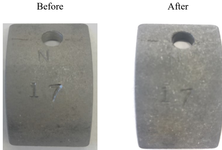
Figure 5.20 Tested steel coupon before and after soaking it at 200°F and 1,000 psi using 27 wt% LA:GA acid mixture solution for 4 hours with 5 gpt of corrosion inhibitor.
