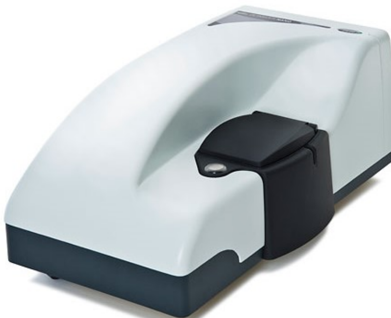
Figure 3.3 A photo of the Zetasizer Nano series used to measure the Zeta potential.
