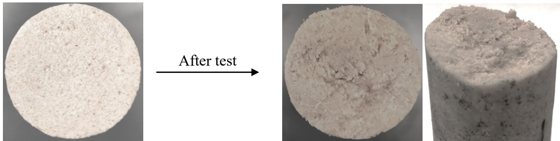
Figure 7.2 Test 1 core inlet face before and after treatment showing face dissolution due to low injection rate.
