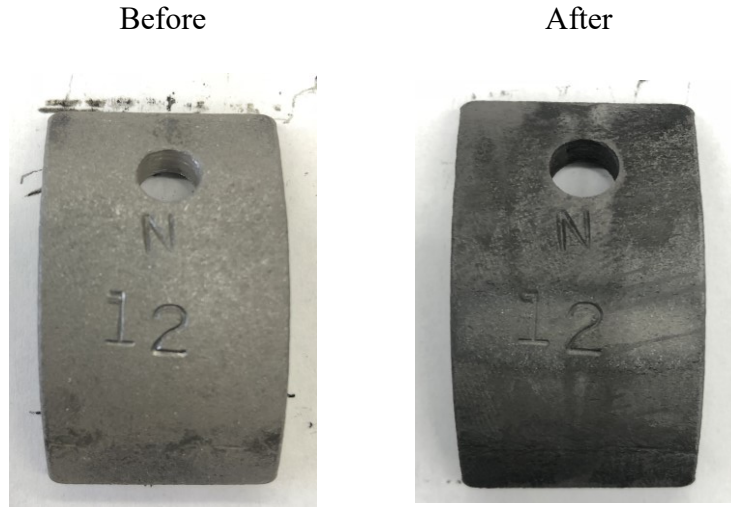
Figure 5.12 Tested steel coupon before and after soaking it at 200°F and 1,000 psi using 14 wt% LA:GA acid mixture solution for 4 hours.
