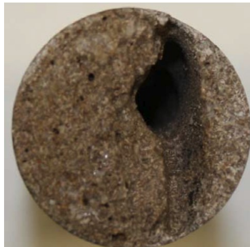
Figure 2.7 A carbonate core that was coreflooded using HCl at high temperature. The high reactivity and dissolving power caused a face dissolution to this core (From Akanni and Nasr-El-Din 2016).
