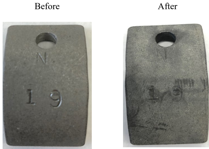
Figure 5.21 Tested steel coupon before and after soaking it at 300°F and 1,000 psi using 27 wt% LA:GA acid mixture solution for 4 hours with 5 gpt of corrosion inhibitor.
