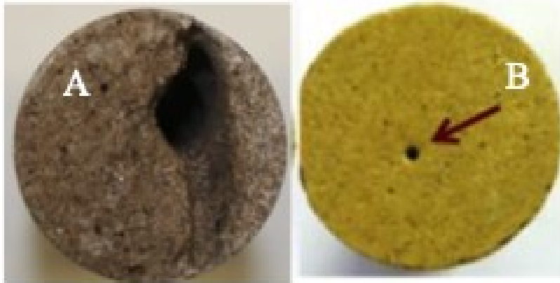
Figure 1.1 Coreflooded cores that represent face dissolution (A) and a dominant wormhole (B) (He et al. 2011; Akanni and Nasr-El-Din 2016).
