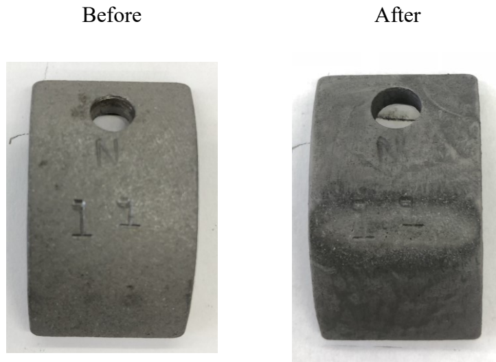
Figure 5.13 Tested steel coupon before and after soaking it at 300°F and 1,000 psi using 14 wt% LA:GA acid mixture solution for 4 hours.
