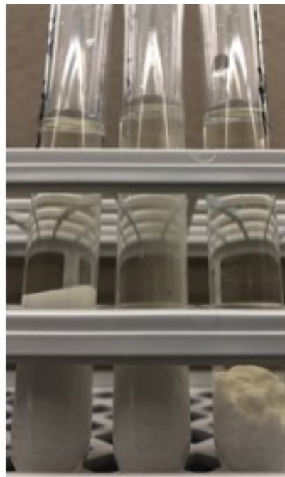
Figure 4.16 Sampling tubes from acids prepared with synthetic seawater that were reacted with crushed core at room conditions. Calcium sulfate precipitation started to appear after a few days of conducting the test.
