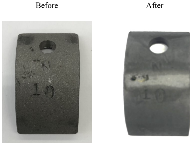
Figure 5.14 Tested steel coupon before and after soaking it at 300°F and 1,000 psi using 27 wt% LA:GA acid mixture solution for 4 hours.
