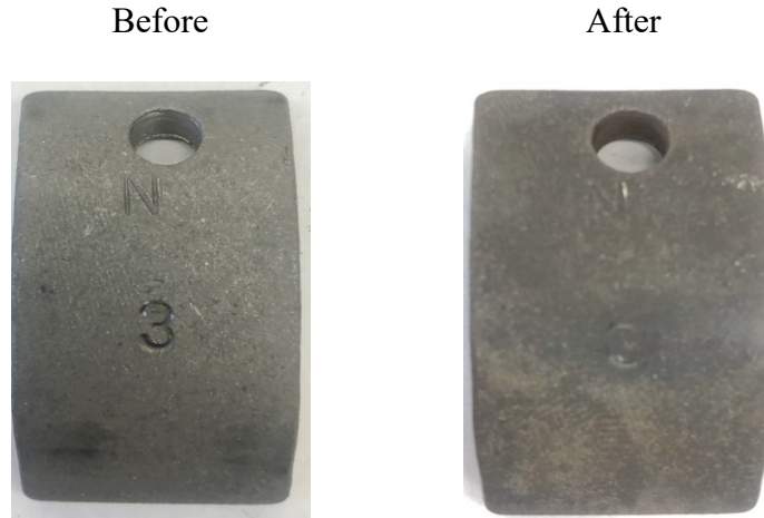
Figure 5.22 Tested steel coupon before and after soaking it at 300°F and 1,000 psi using 27 wt% LA:GA acid mixture solution for 12 hours with 5 gpt of corrosion inhibitor.
