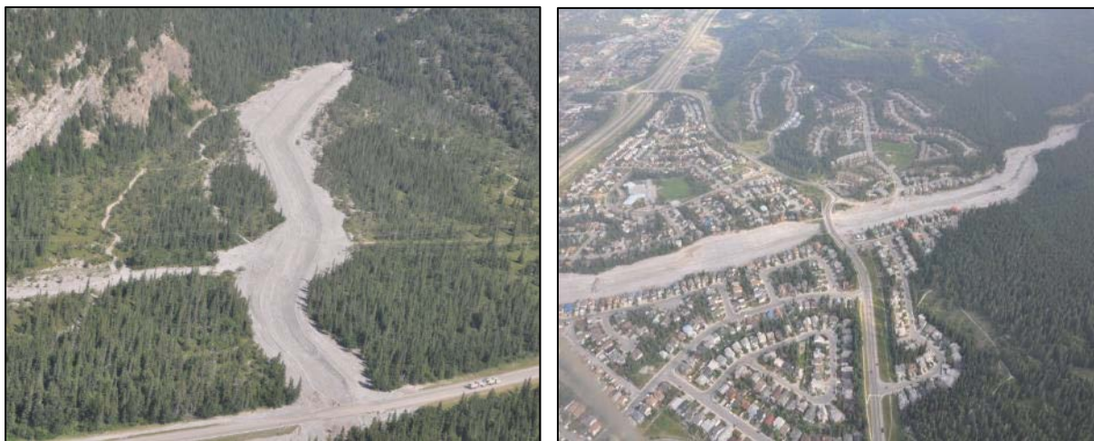
Fig 2. An undeveloped fan (left) and a highly-developed fan (right) in Alberta, Canada, both prone to debris floods. A prescriptive standards-based process would call for the same design event (100 or 150 years in the case of Switzerland, Japan or Austria) for mitigation for each fan. The QRM process would prescribe a relatively small structure for fan A, and a major structure or series of structures for fan B.
