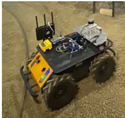
Figure 3.2 Husky robot for data collection in Edgar Mine
