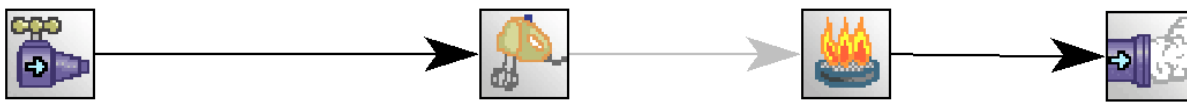
Figure 2.7 PREMIX simulation schematic in Chemin with an inlet source, non-reactive mixer, premixed laminar burner-stabilized flame, and outlet flow models (from left to right).
