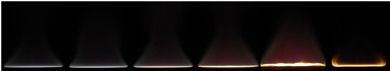
Figure 2.4 Photographs of \text{H}_2/\text{NH}_3 flat flames ranging from 70% \text{H}_2 on the left to 20% on the right in 10% increments. The ideal flat flame condition is lost in the last 2-3 images. Reprinted from Ref. [30], an open source presentation.
