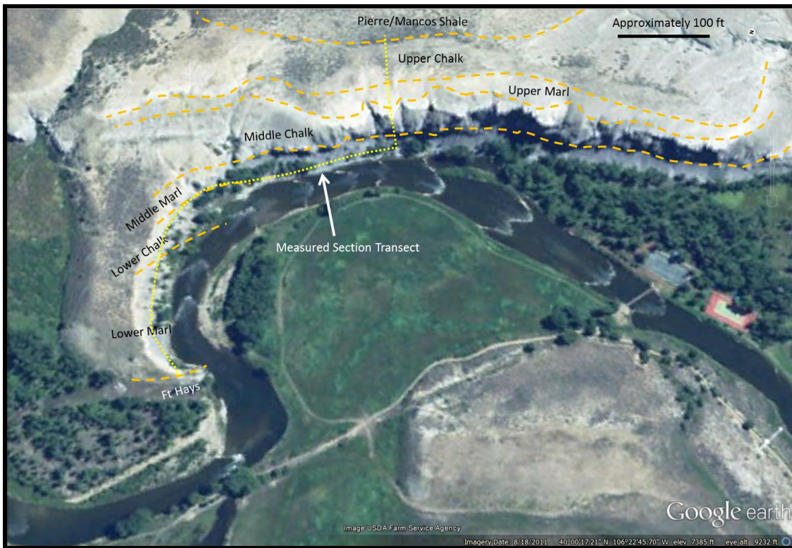
Figure 3.4B Google Earth image showing the measured section transect for Fort Hays through the Upper Chalk at Kremmling along the Blue River located in section 32-T1N-R80W.
