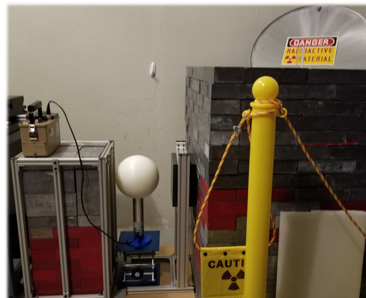
Figure 1: The experiment setup. From left to right: beam stop, neutron detector, borated blocks and cylinders, radioactive source and container.
