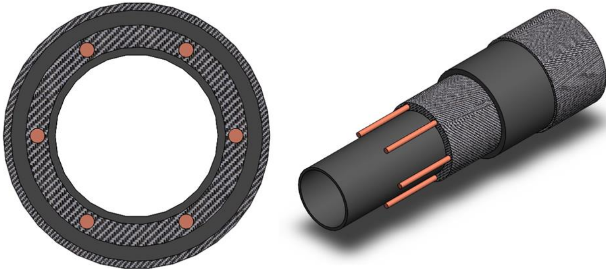
Figure 1.2: Conceptual rendition of a piece of composite coiled tubing. The left figure represents a cross section, and the right demonstrates the layers.
