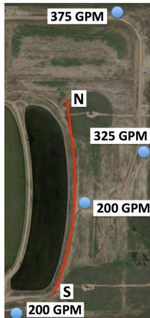
Figure 3.30: Electrical resistivity tomography survey location (red line) with the steady recovery well pumping rates (in GPM) during the measurement period.
