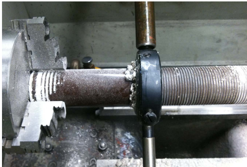
Figure 3.20: Threading epoxy fiberglass rods by hand requires the use of a lathe to hold the epoxy fiberglass rod in place while one to two people use lever arms to turn the die quarter turns at a time with brute force, which can boil lubricant and burn epoxy fiberglass.
