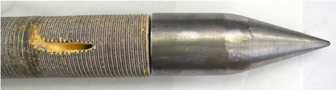
Figure 3.23: The bottom of a recovered high-resolution temperature sensing probe, where the fiber-optic cable does not exceed the critical bend angle and is protected with epoxy resin. The cable exits through the curved trough, slit, and up through the inner rod core. (Not original drive point).
