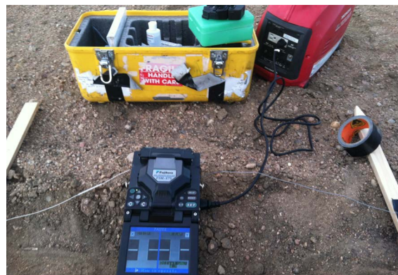
Figure 3.24: The Fujikura arc-fusion splicer utilizes a microscope to image splices and then references a library of splice images with known optical losses of light (in dB) to estimate the optical loss due to the splice. Splices for the high-resolution temperature sensing probe array were only accepted with estimated 0.0 dB losses.
