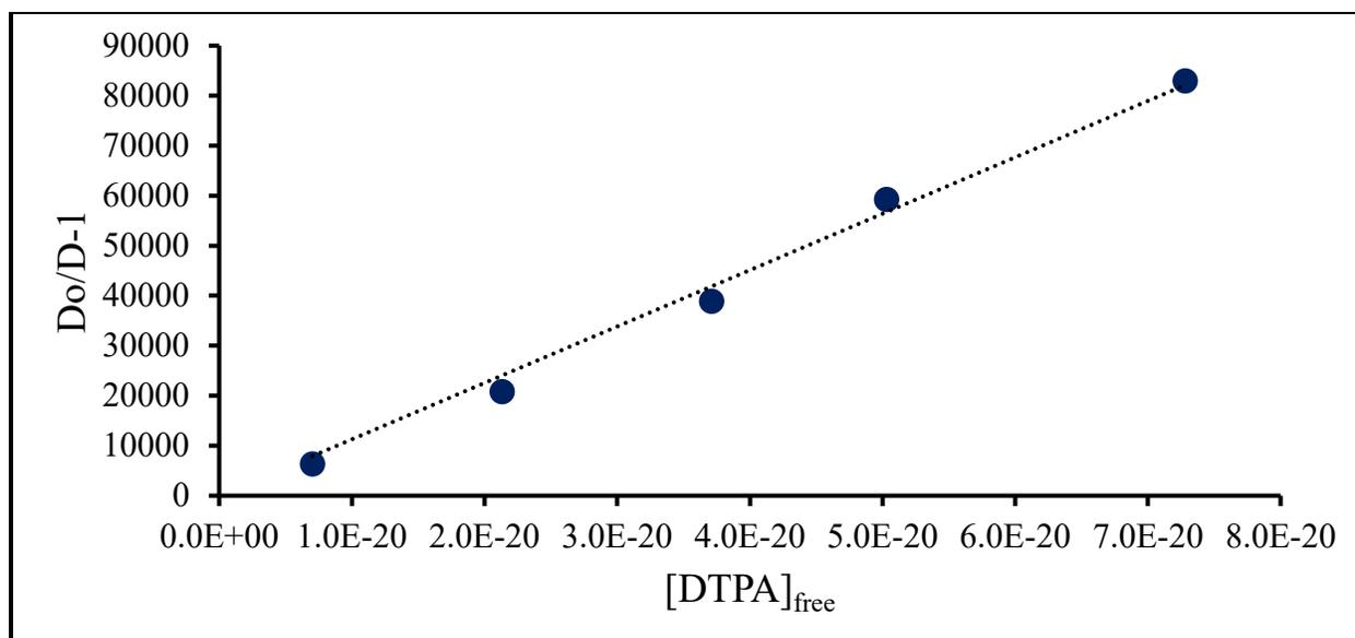
Figure D.88: Fit of Es-DTPA T = 25°C, pcH = 2.3 data
