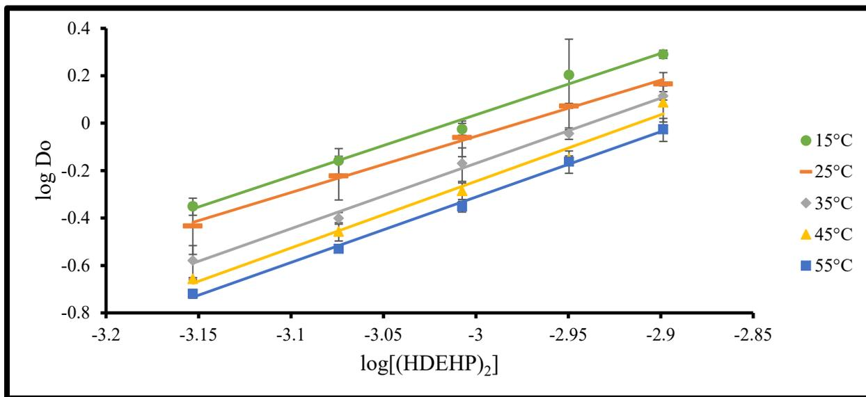
Figure 4.2: Results of berkelium equilibrium extraction trials,  $I = 0.5 \text{ M}$ ,  $\text{pH} = 2.5$ .
