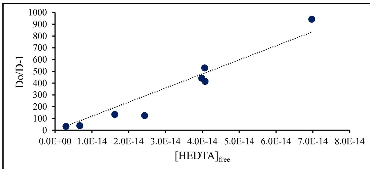
Figure D.48: Fit of Cf-HEDTA T = 25°C data
