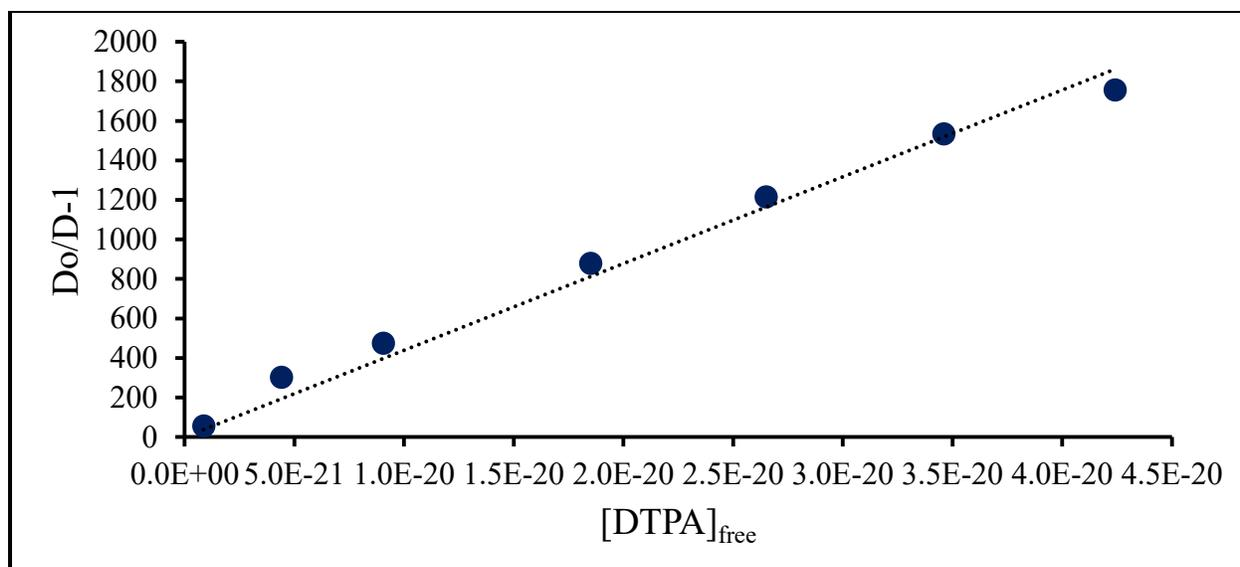
Figure D.30: Fit of Bk-DTPA T = 35°C, pcH = 2.1 data
