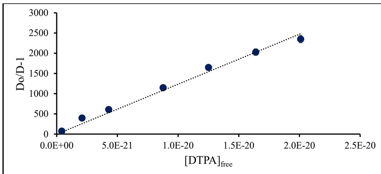
Figure D.26: Fit of Bk-DTPA T = 25°C pcH = 2.1
