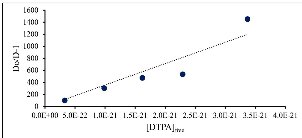
Figure D.93: Fit of Es-DTPA T = 35°C, pcH = 1.9 data
