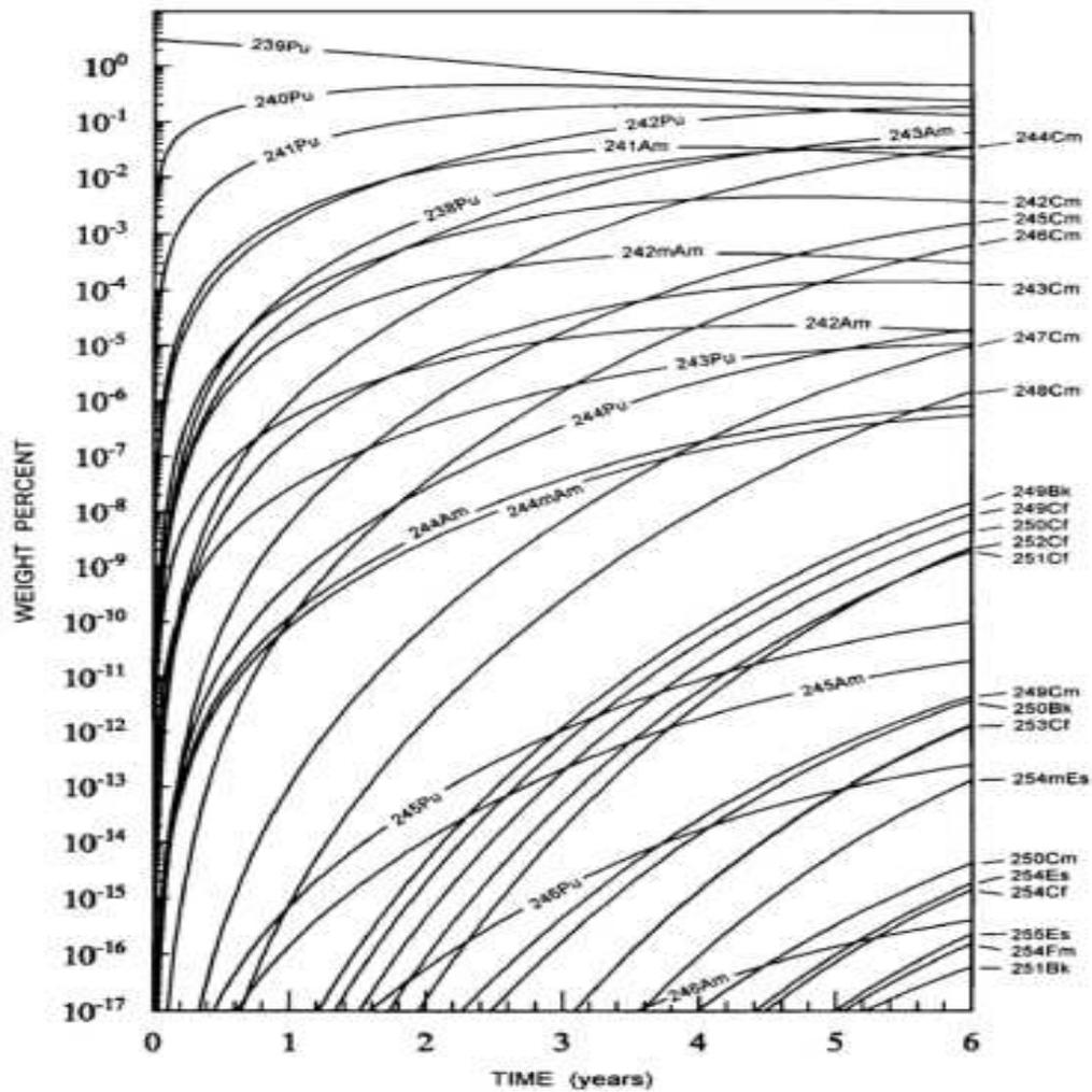
Figure 2.2: Weight percent of transuranic isotopes produced in MOX fuel as a function of time in a thermal spectrum reactor. As fuel is recycled continuously, production of these isotopes increases. These trace isotopes may cause problems in controlling a thermal reactor as many are either neutron absorbers or decay via spontaneous fission, releasing neutrons and affecting the neutron economy of the reactor (Choppin et al., 2001).
