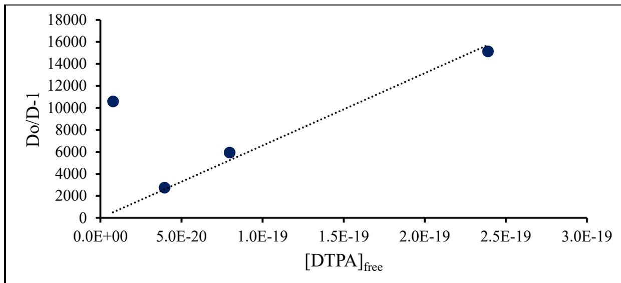
Figure D.40: Fit of Bk-DTPA T = 55°C, pcH = 2.3 data
