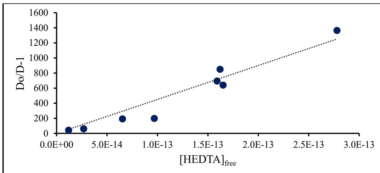
Figure D.51: Fit of Cf-HEDTA T = 55°C data
