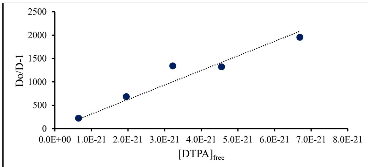
Figure D.96: Fit of Es-DTPA T = 45°C, pcH = 1.9 data
