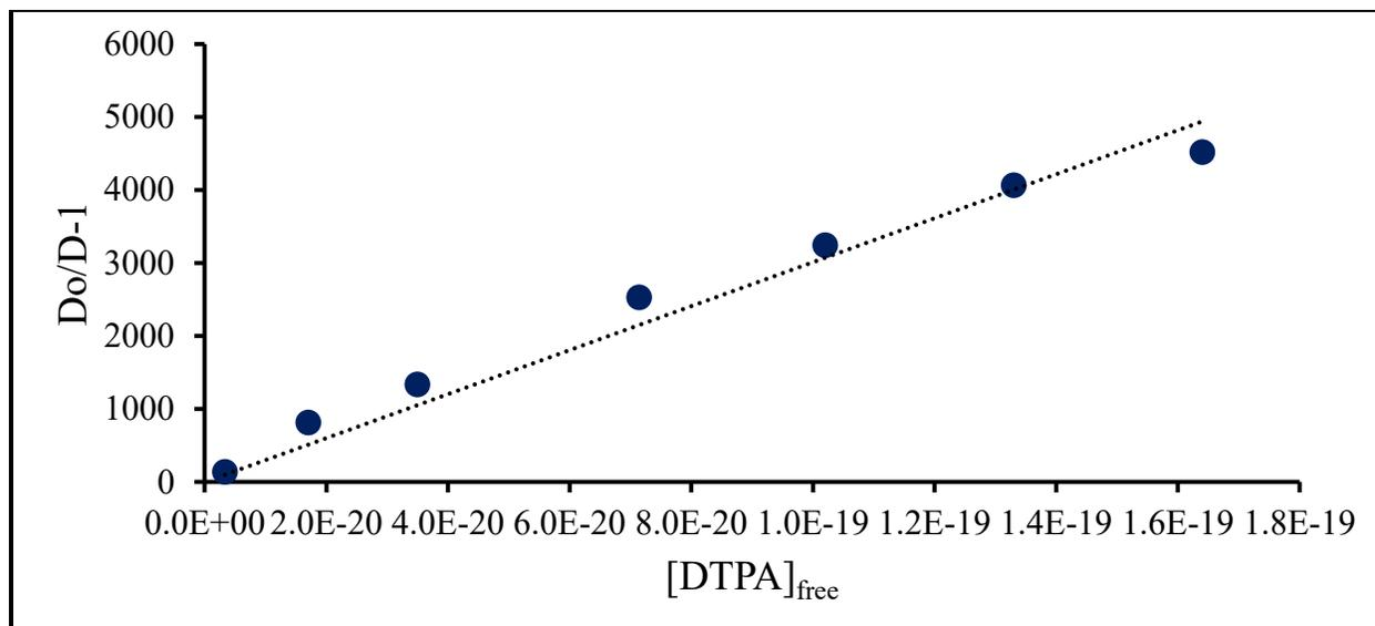
Figure D.38: Fit of Bk-DTPA T = 55°C, pcH = 2.1 data
