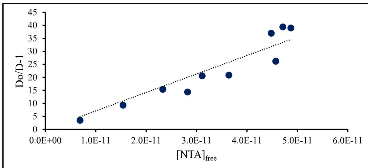
Figure D.14: Fit of Bk-NTA T = 45°C data
