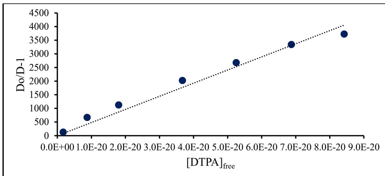
Figure D.34: Fit of Bk-DTPA T = 45°C, pcH = 2.1 data
