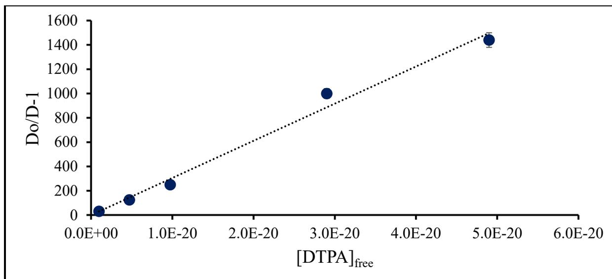
Figure D.28: Fit of Bk-DTPA T = 25°C, pcH = 2.3
