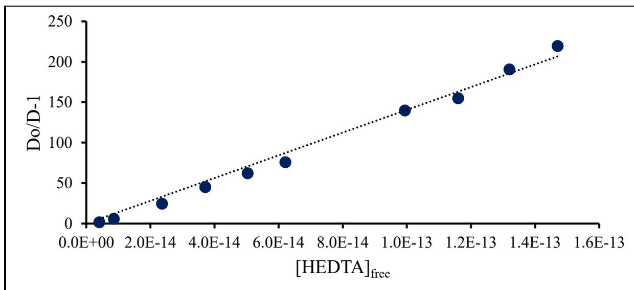
Figure D.19: Fit of Bk-HEDTA T = 45°C data
