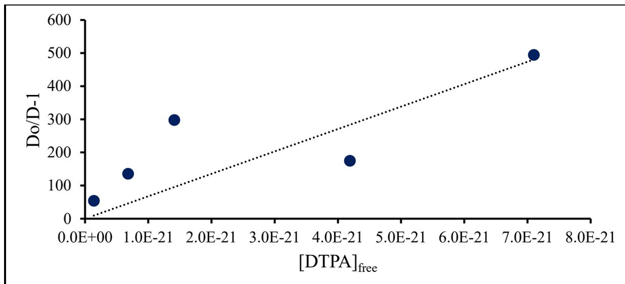
Figure D.35: Fit of Bk-DTPA T = 45°C, pcH = 1.9 data
