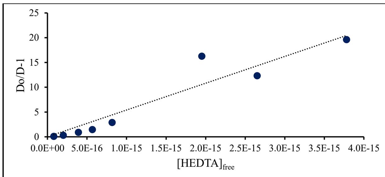
Figure D.10: Fit of Am-HEDTA T = 55°C data
