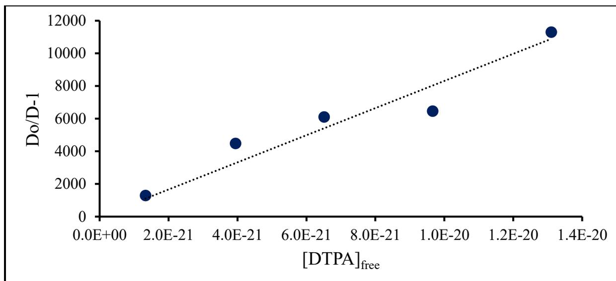
Figure D.89: Fit of Es-DTPA T = 25°C, pcH = 2.1 data
