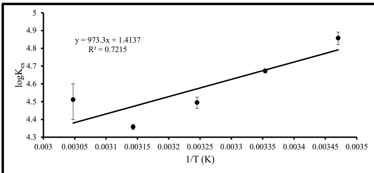
Figure A.3: Californium extraction Van't Hoff plot
