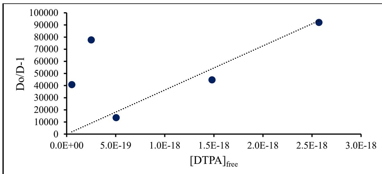
Figure D.41: Fit of Bk-DTPA T = 55°C, pcH = 2.5 data
