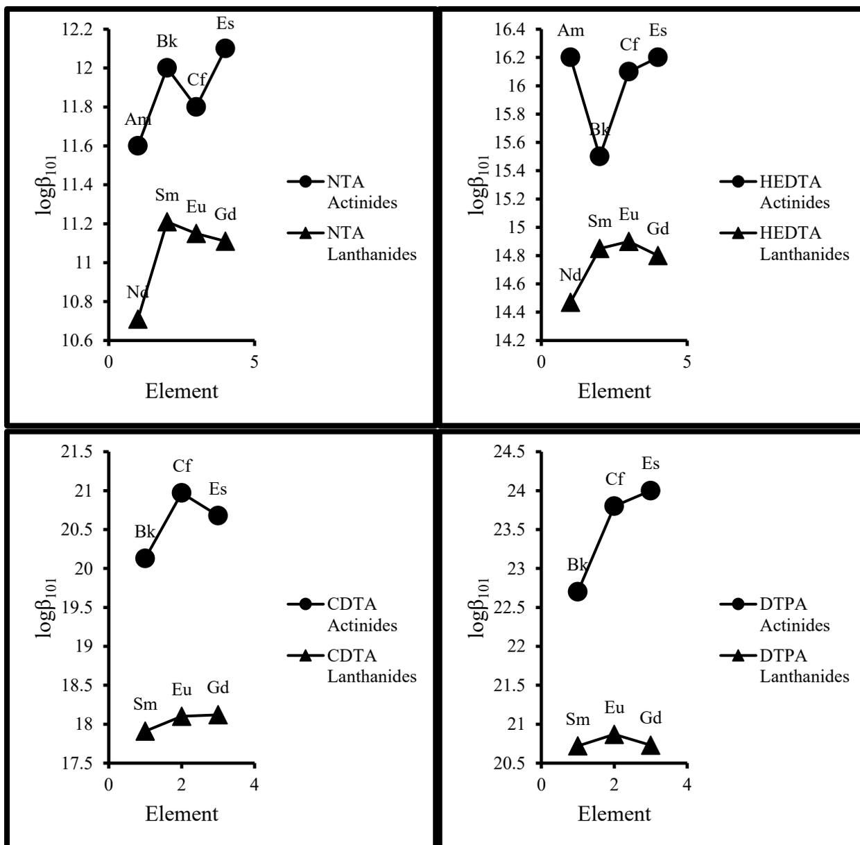
Figure 5.19: Comparisons between APC stability constants for actinides and lanthanides. CDTA and DTPA Am and Nd constants omitted.
