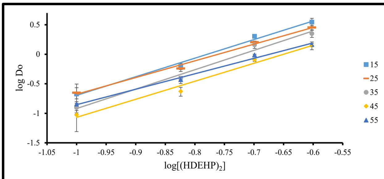
Figure 4.4: Results of einsteinium equilibrium extraction trials,  $I = 0.5 \text{ M}$ ,  $\text{pH} = 2.5$ .
