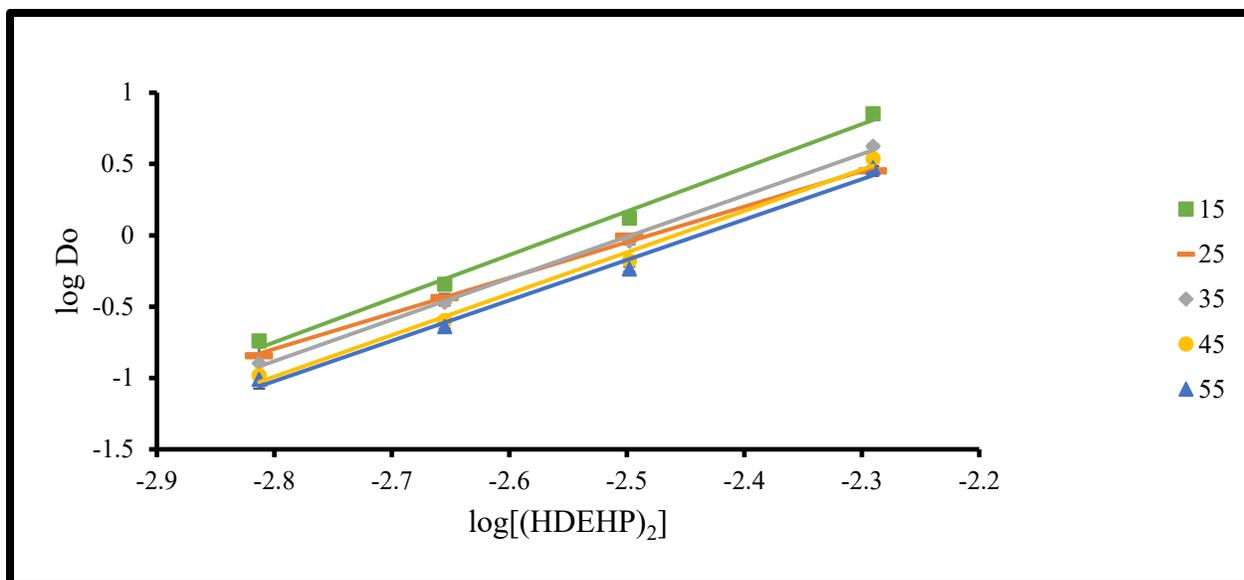
Figure 4.1: Results of americium equilibrium extraction trials,  $I = 0.5$  M,  $p\text{cH} = 2.5$ , HDEHP in n-dodecane.
