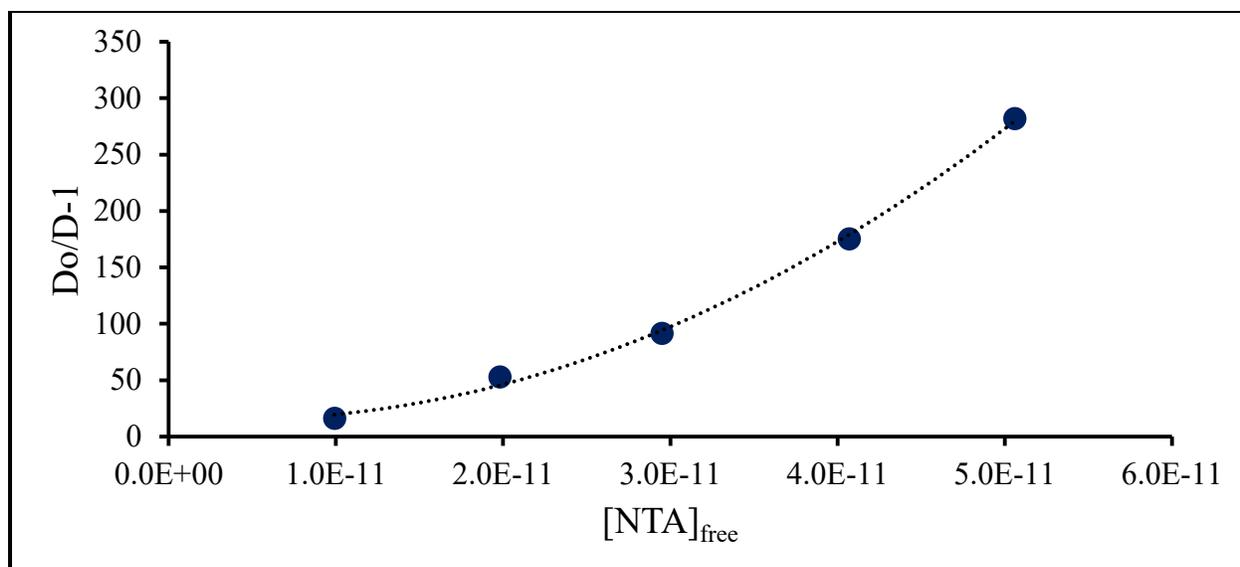
Figure D.74: Fit of Es-NTA T = 25°C data
