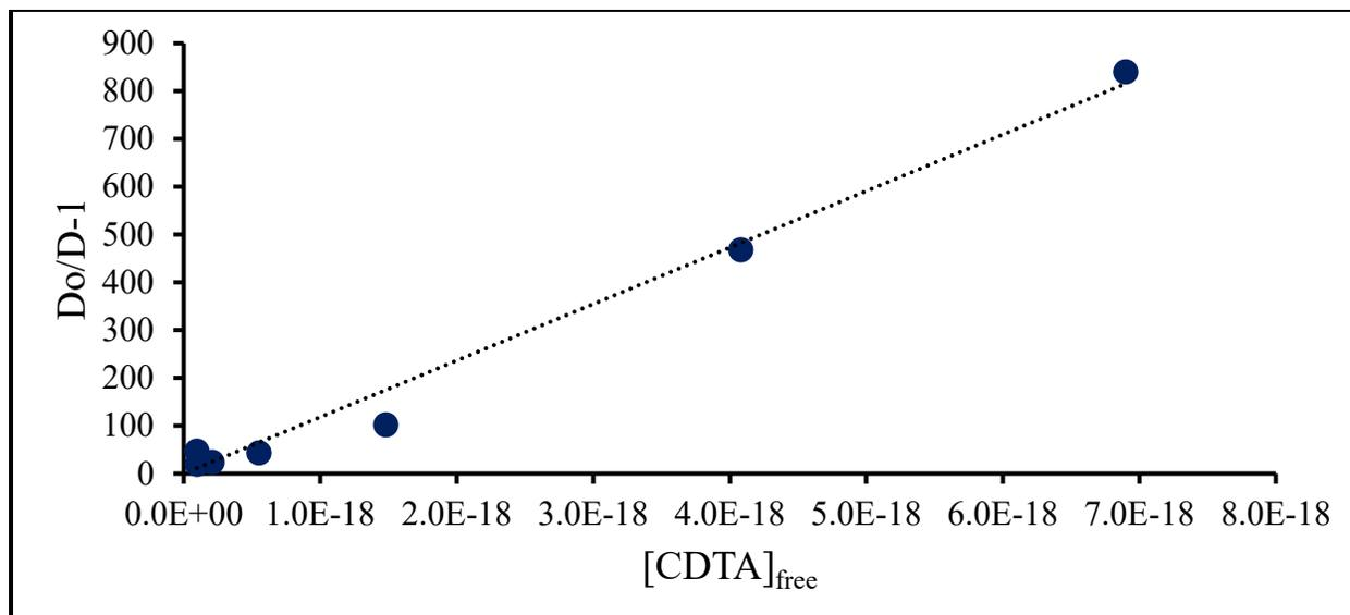
Figure D.22: Fit of Bk-CDTA T = 30°C data
