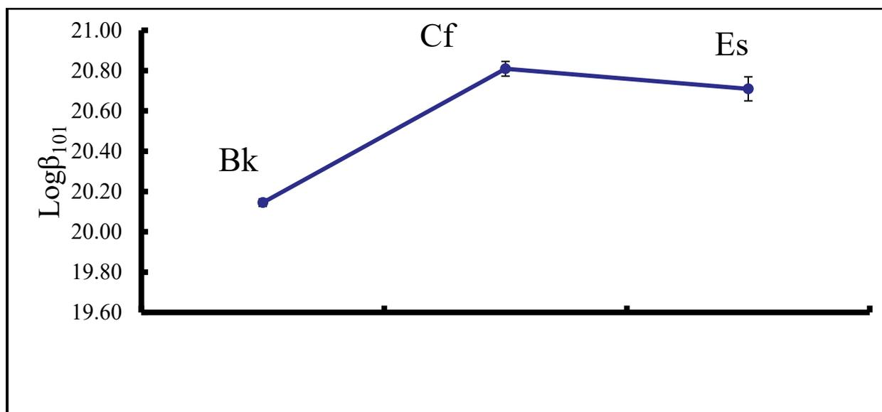
Figure 5.10: Stability constant trend for An-CDTA
