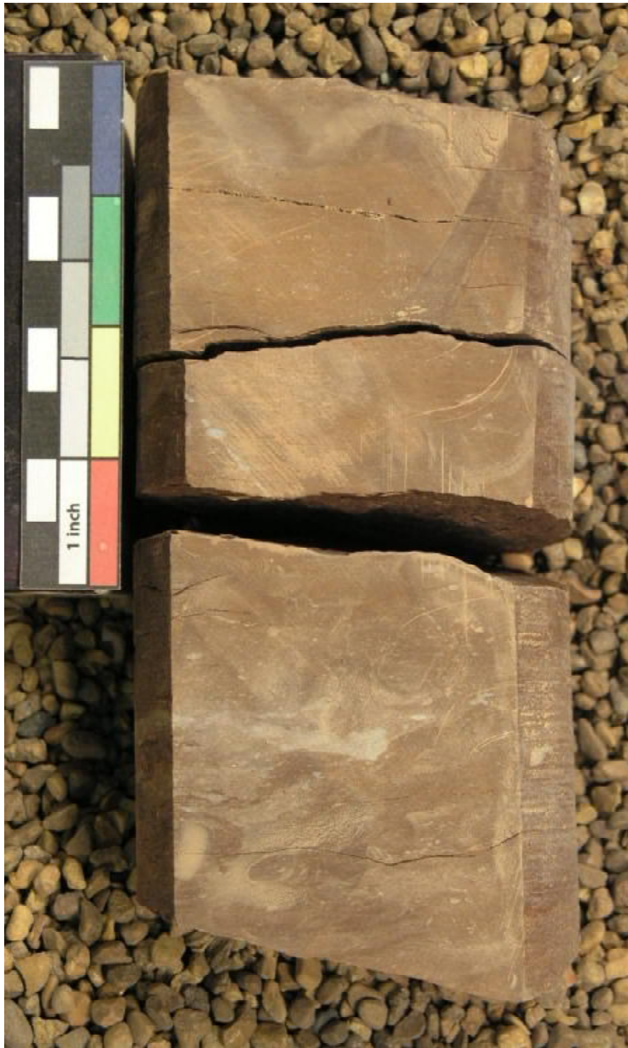
Figure 3.3. Facies A. Core #2. 10,701 feet. Facies A consists of moderate red (5 R 4-6) to pale red (5 R 6-2) dolomitic shale with white dolomite clasts.
