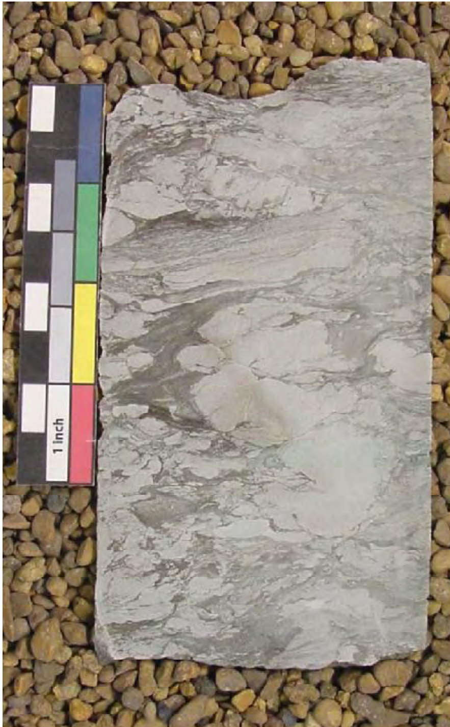
Figure 3.5. Facies C. Core #1. 10,333 feet. Facies C is dominated by soft-sediment deformation and brecciation. Facies C is a light green (5 G 8-1) to greenish-gray (5 G 6-1) shale mixed with light gray silty dolomite (N8).
