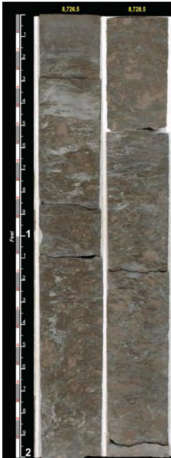
Figure 3.24. Core #16. 8,726.5 to 8729.5 feet. Facies C in northern North Dakota. Used with the permission of Samson Resource.
