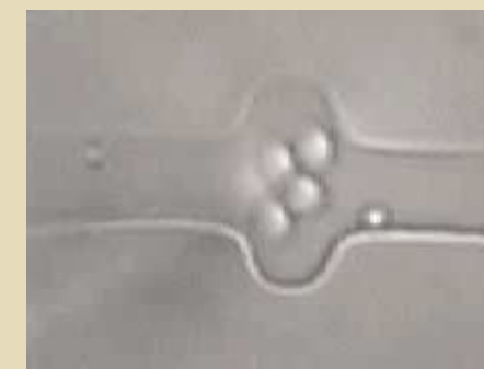
A gear pump created from colloidal particles is the size of a red blood cell.
