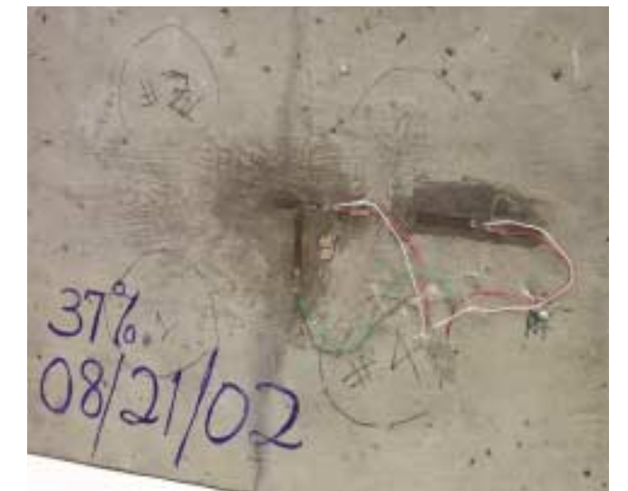
Results show composite concrete (with 37% replacement of aggregates) after an identical explosive charge.
