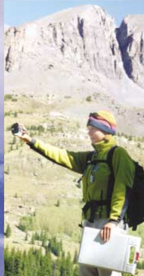
▶ Geology student Robyn Brown uses a Brunton compass to measure the thickness of sedimentary rocks during field session near Silverton, Colo.
