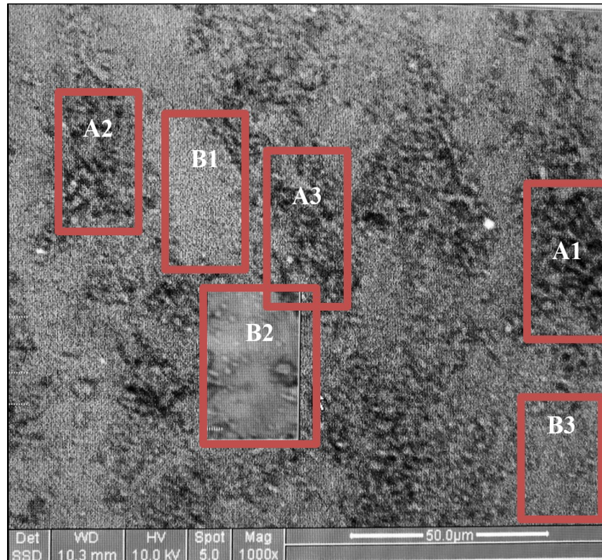
Figure 4.5: The features on unpolished Niobrara sample. Note the poor quality of image is due to obtaining the image from ESEM and low accelerating voltage.
