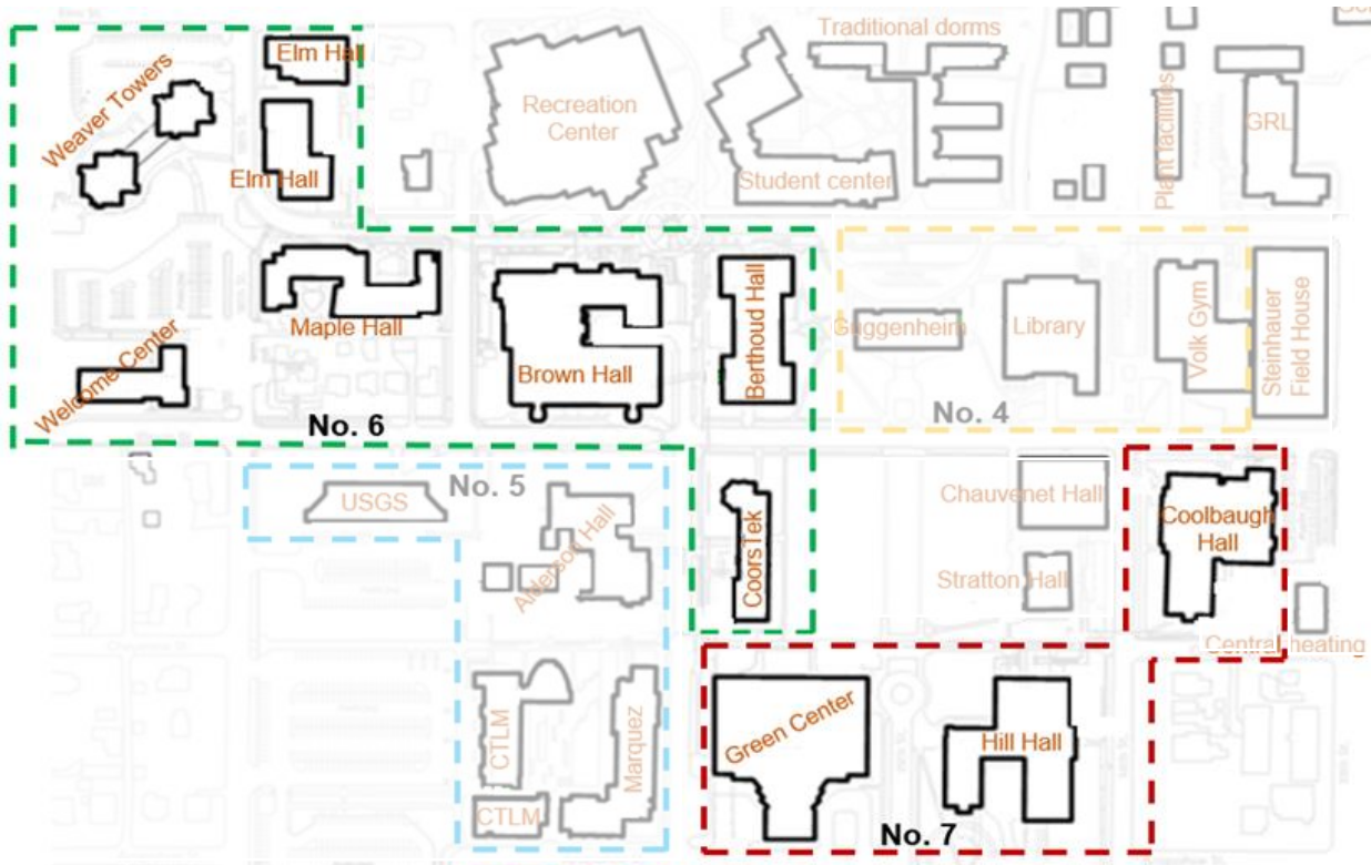
Figure 7-5: Colorado School of Mines main campus with chiller loops 6 and 7 marked in green and red, respectively [132]
