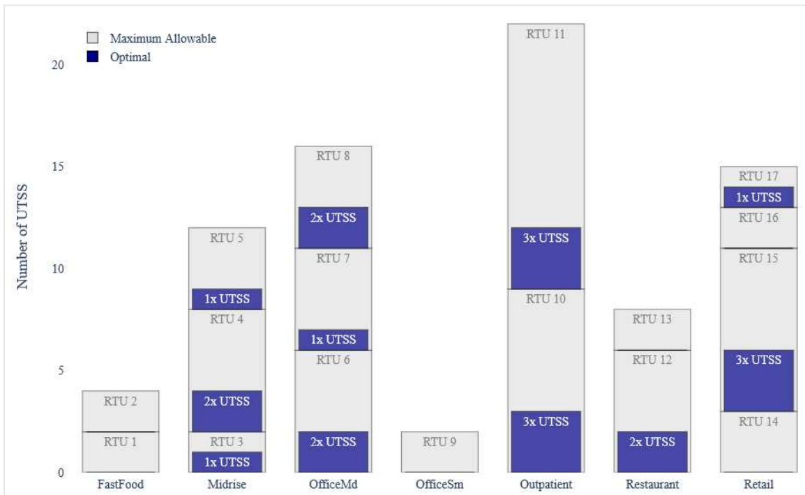
Figure 6-6: Optimal UTSS placement by RTU, grouped by building. Each gray box depicts the maximum number of UTSS that could be assigned to given RTU, which is equivalent to the parameter m_{in} . The blue boxes depict the number and location of UTSS given by the optimized solution.
