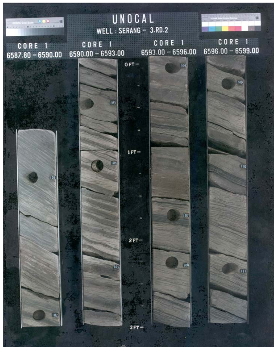
Figure 4.13: Fluvial/distributary channel sandstone with 60 API gamma ray readings at 6596 ft is used as sandstone cut-off in calculating net sand in this study. This sandstone has higher mud content compared to the sandstones below it. The sandstones above 6596 ft are more mud-prone compared to those below 6596 ft.
