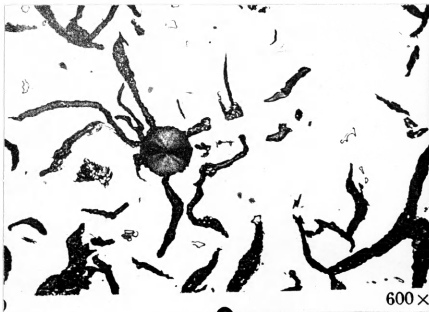
Fig. 1 - Graphite Nodule Obtained by Hanemann by Treating Cast Iron with Titanium Carbide
