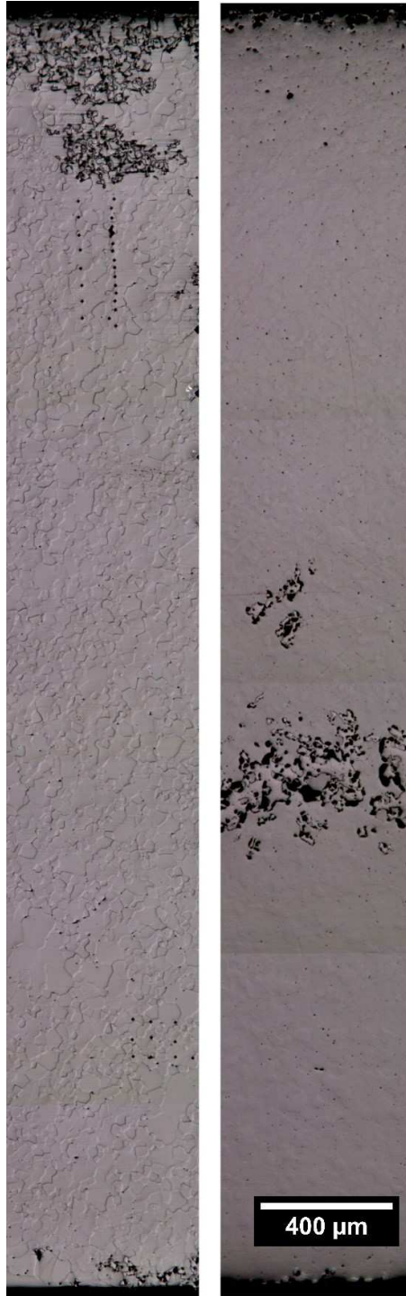
Figure 3.7 Polished cross sections of two specimens are shown. Material that was HIPed, then heat treated in air at 1573 K for 10 hours (left) is compared to material that was HIPed, then heat treated in air at 1873 K for 24 hours, then heat treated in vacuum at 1573 K for 10 hours (right), demonstrating that precipitation can occur at the surface or at the core depending on processing conditions.
