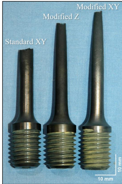
Figure 3.6. Comparison of deformation in 145 MPa creep samples of standard Haynes 230 (XY-oriented), modified Haynes 230 (XY-oriented), and modified Haynes 230 (Z-oriented).
