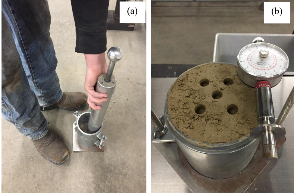
Figure 6.13 Compaction and UCS measurement using: (a) Proctor compaction; and (b) Penetrometer.
