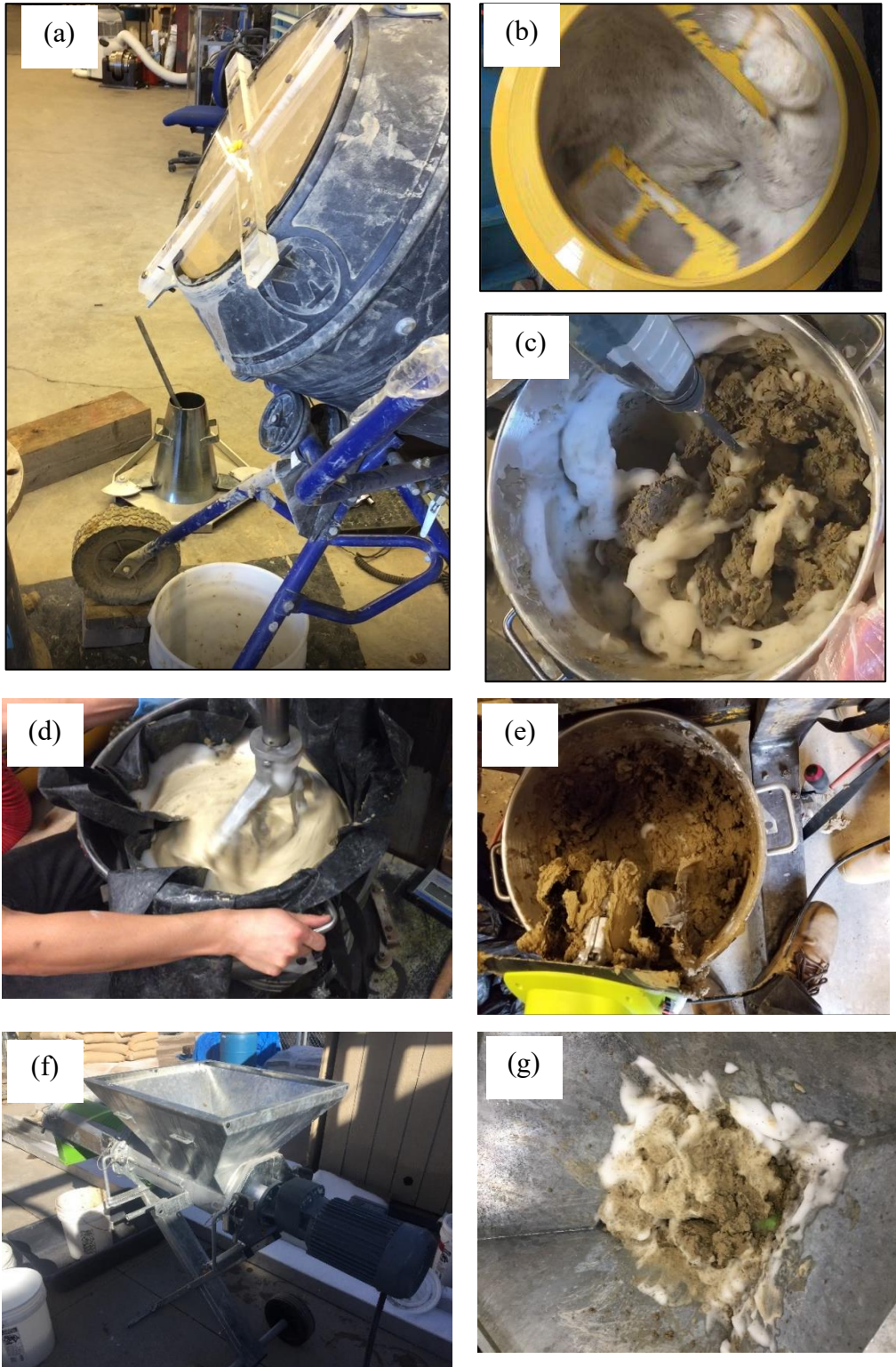
Figure 6.3 Tools for mixing Denver clay and foam: (a) and (b) concrete mixers; (c) a hammer drill mixing tool; (d) a flat beater with the rheometer power; (e) a tiller mixer; (f) a continuous mixer; and (g) clogged clay in the continuous mixer.
