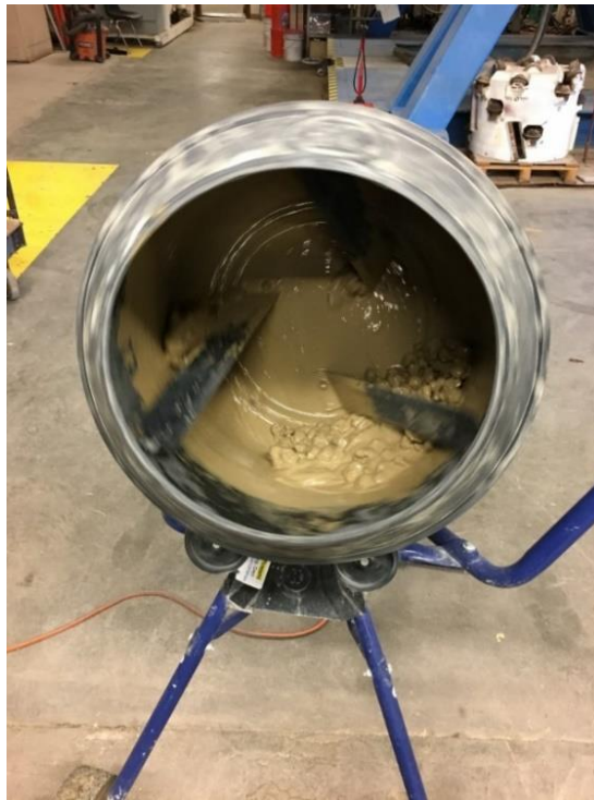
Figure 4.5 A concrete mixer used to mix CSM sand and water.
