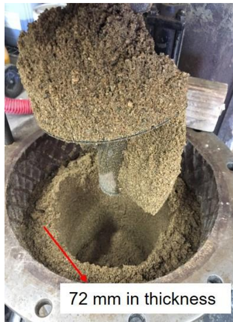
Figure 5.11 Gap between the outer edge of the small auger and the chamber wall.
