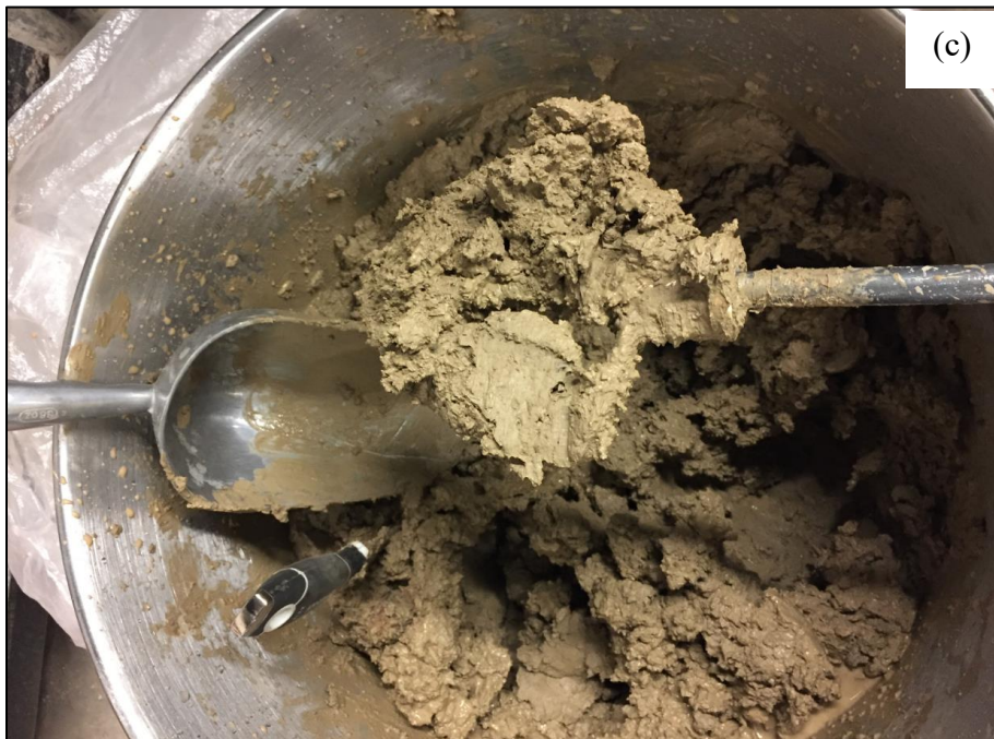
Figure 6.2 Tools for mixing Denver clay and liquid: (a) a concrete mixer; (b) a dough mixer; and (c) a hammer drill mixing tool.
