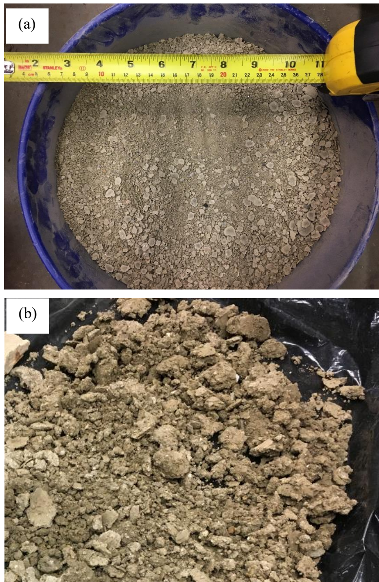
Figure 6.1 Denver clay before mixing: (a) pulverized clay powder; and (b) clay lumps.
