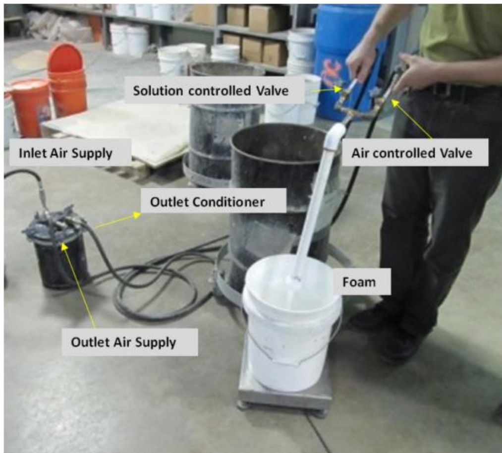
Figure 5.6 Foam generator in this study (Alavi, Rostami, and Talebi 2014).
