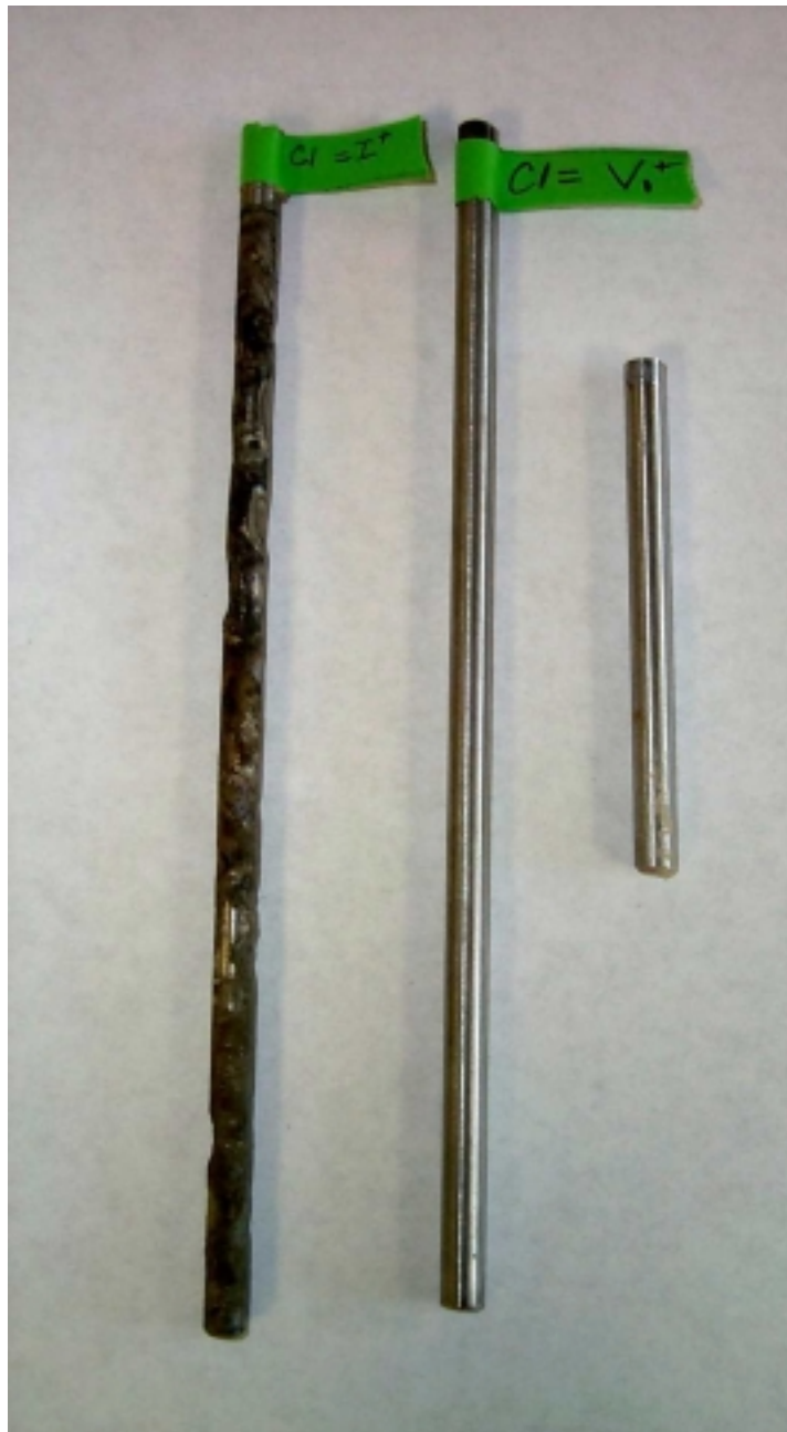
Figure 5.34. One current electrode (left) and one potential electrode (middle) removed from column 1, the high-grade ore with biooxidant , on 3/3/99. The raw MP35N (right) looks identical to the potential electrode.
