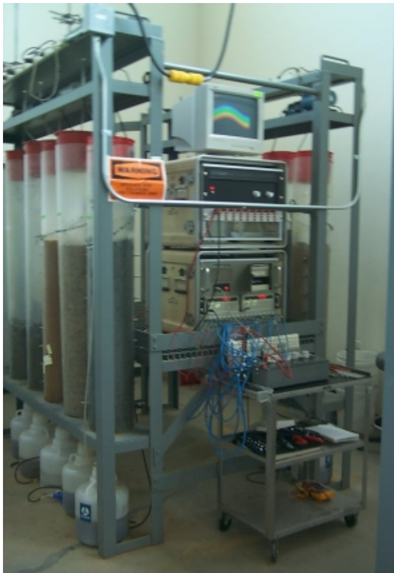
Figure 4.5. The set-up of columns and CR equipment at Newmont in Englewood, CO. This picture shows the test of all channels across decade resistor boxes, one for the potential channels and one for the current-sensing resistor.
