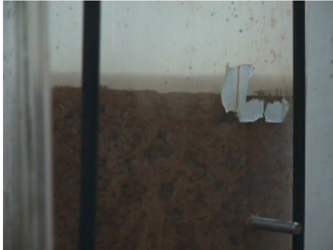
Figure 4.7. Pooling of approximately 1/3 inch of water on the top of the ore in Column 3 near the end of the experiment.
