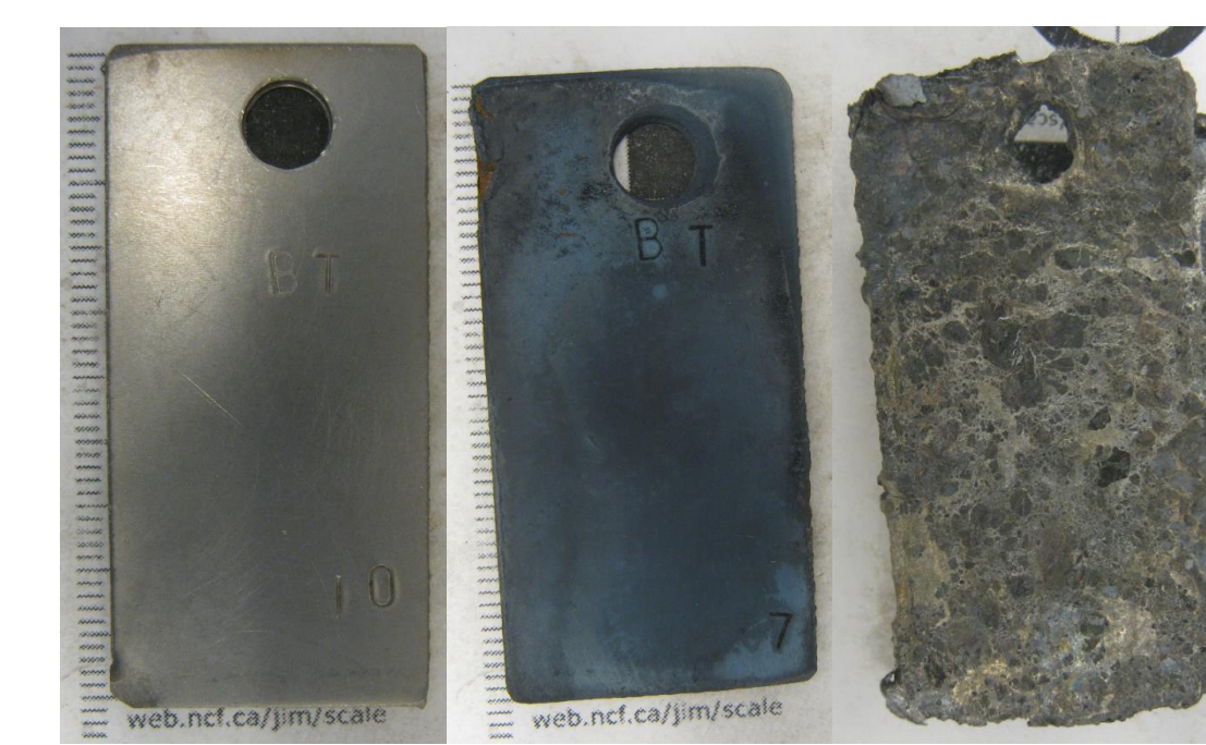
Figure 4: Left to right: virgin titanium, titanium exposed to N2 at 700 C for 200 hours, titanium exposed to molten aluminum at 700 C for 200 hours. The rightmost sample demonstrates the aggressive corrosion of molten aluminum.
