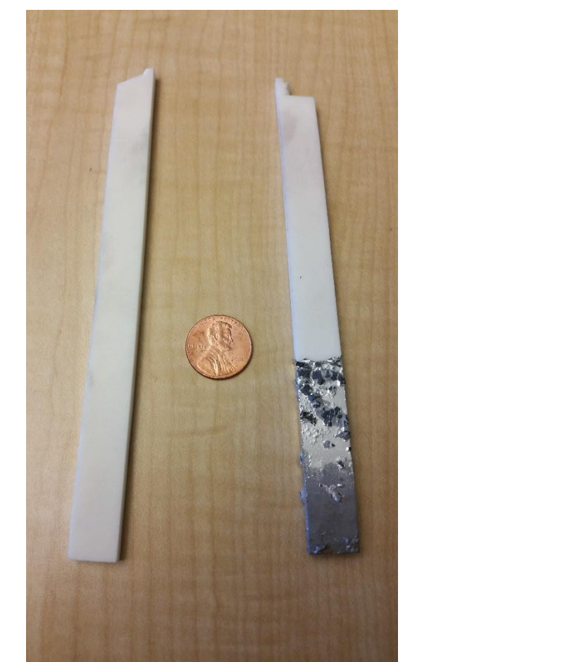
Figure 12: Virgin monolithic aluminum oxide on left and monolithic aluminum oxide on right after 650 hours in molten aluminum 4047 alloy. This combination is currently the most promising candidate and work is currently underway to test stainless steel coated with aluminum oxide.
