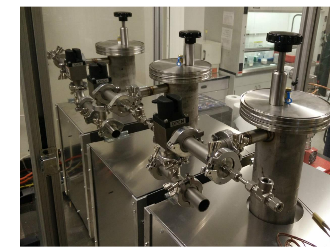
Figure 6: Custom-built furnaces used for molten PCM corrosion testing. Coupon holders are placed into the flanges and then coupons lowered into molten PCM.
