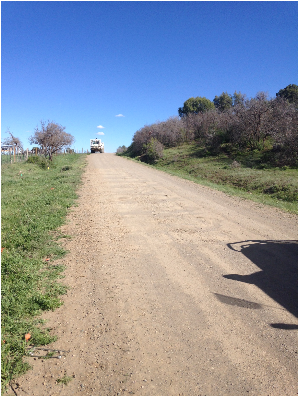
Figure 2.6: Marks on the road indicating the position of Vibroseis plate for experiment B. The distance between consecutive shot location is on the order of 1-2m.
