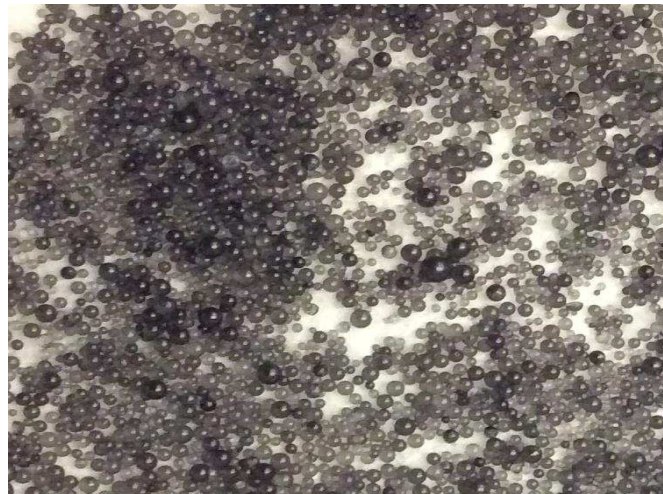
Figure 2.5 FracBlack HT ULW proppant, 14/40 mesh.
