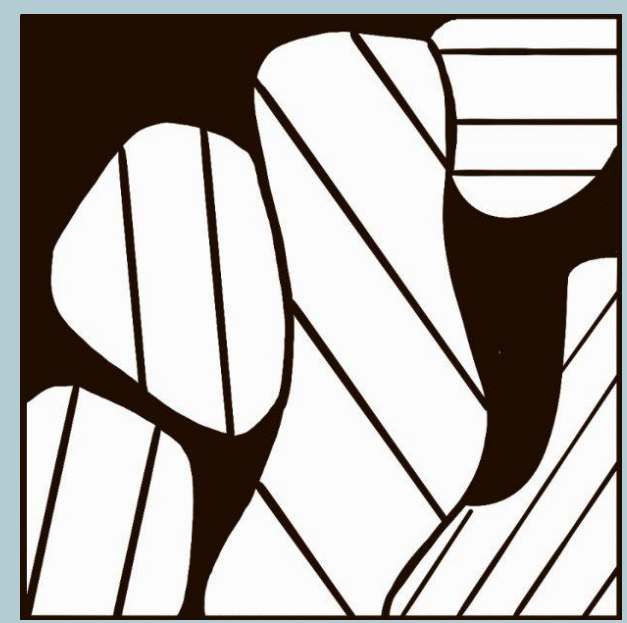
Figure 2: Simplified slip bands, hand generated for initial programming efforts
