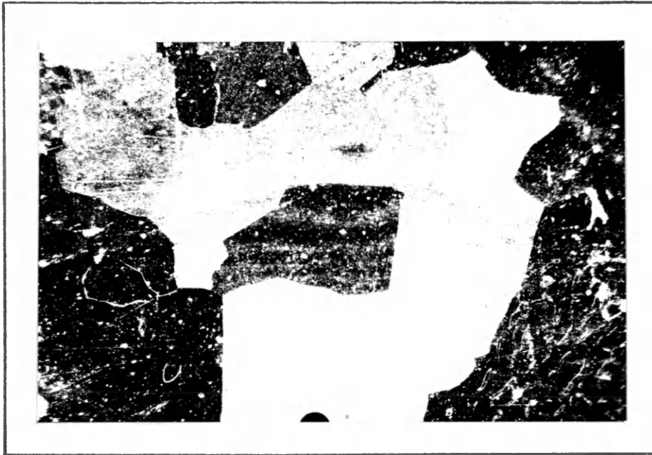
Magnification: 100X Etchant: Ferroxyll indicator containing KCN Time: 5 days Oblique illumination
