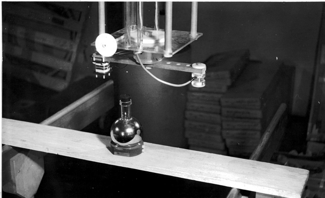
Plate 2 - Source-coil, receiver-coil, and reference-coil over 500 ml mercury sphere
