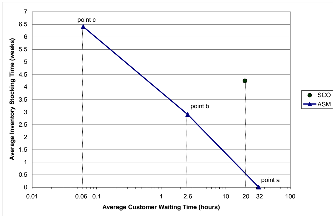
FIG. 5.9. The average time a part spends in inventory versus the average time a customer waits for a part (linear / log scale)
