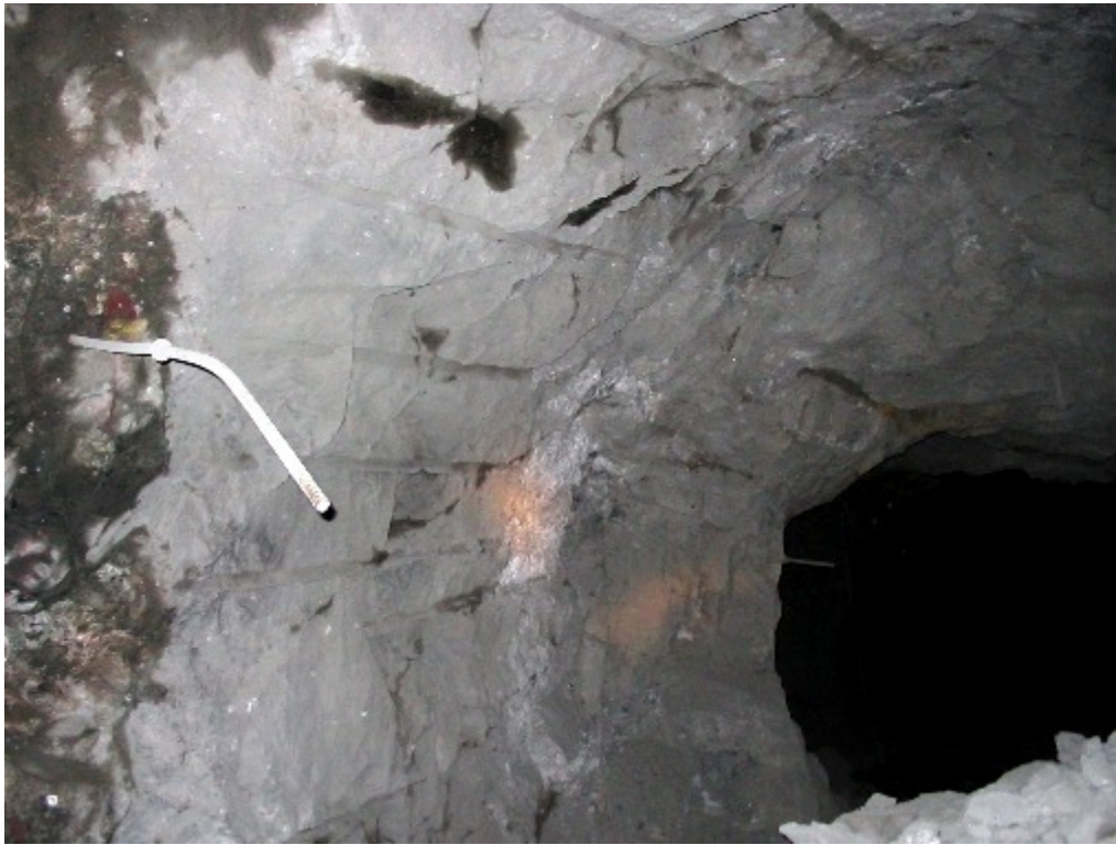
Figure 6.29 Half-cast drill holes visible after blast
