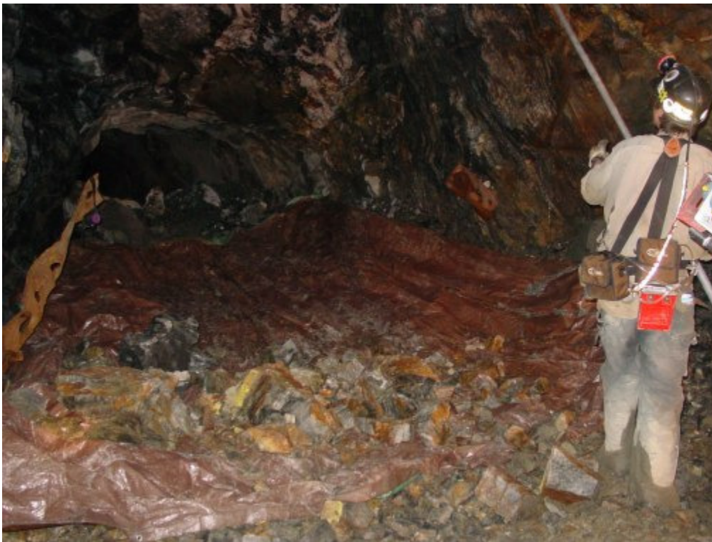
Figure 6.46 Manual scaling during Experiment #9
