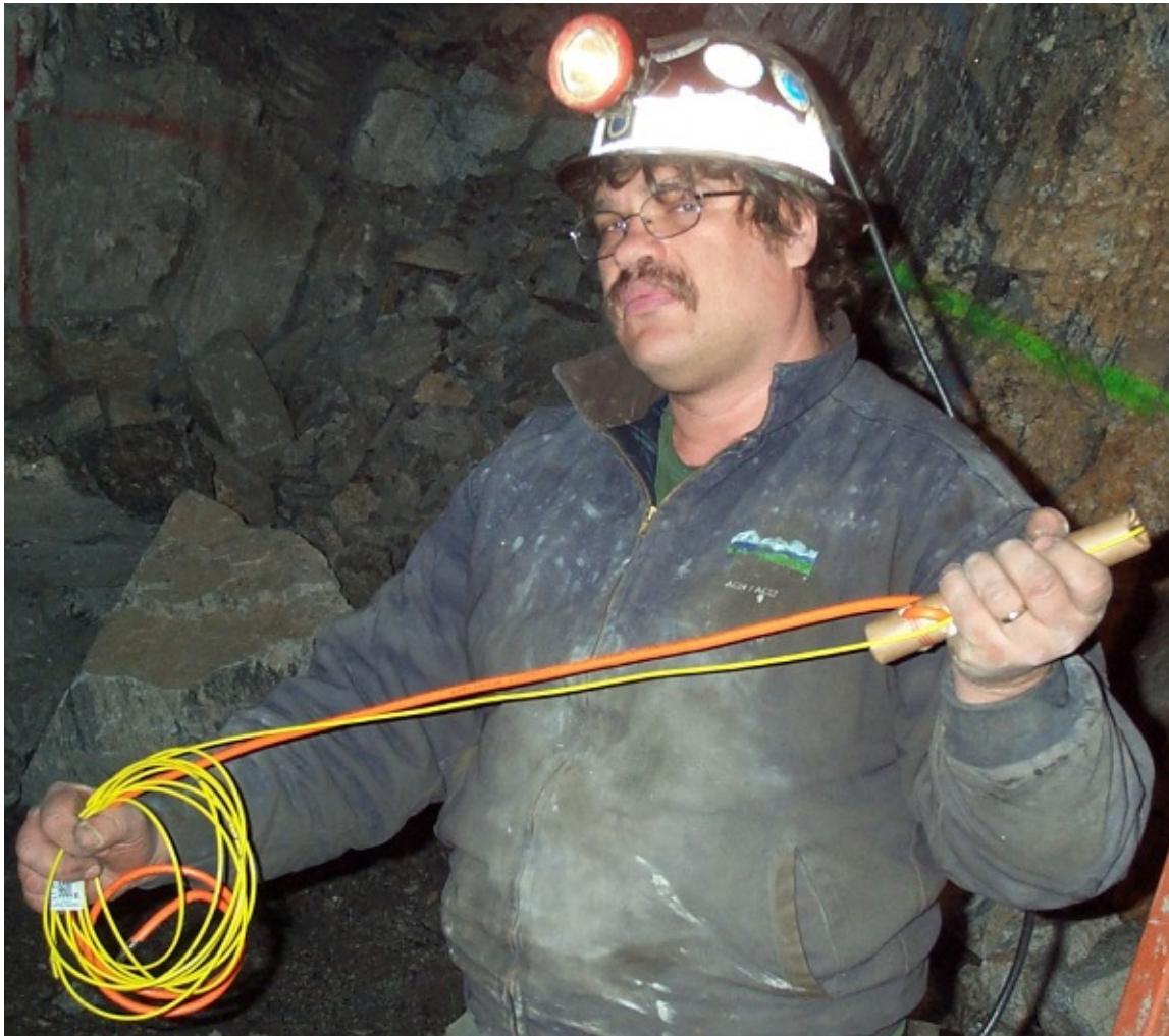
Figure 4.12 Stick of emulsion primed with an 8-gram blasting cap and attached to a 200-grain detonating cord
