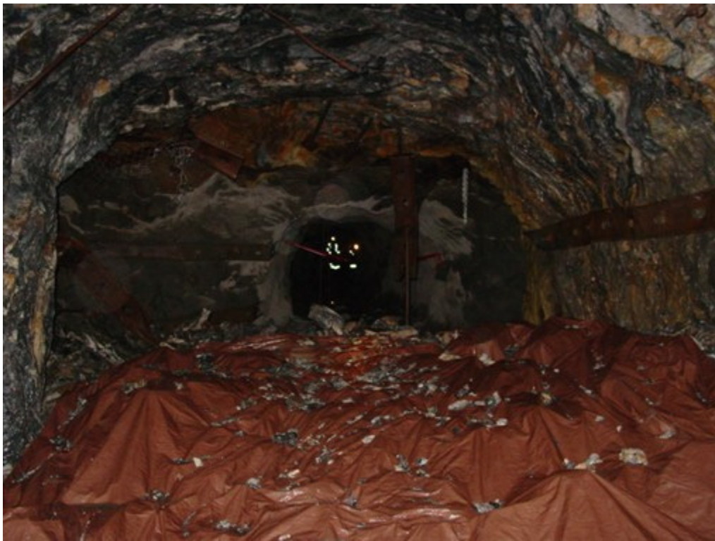
Figure 6.35 Material removed in Experiment #7 waterjet test
