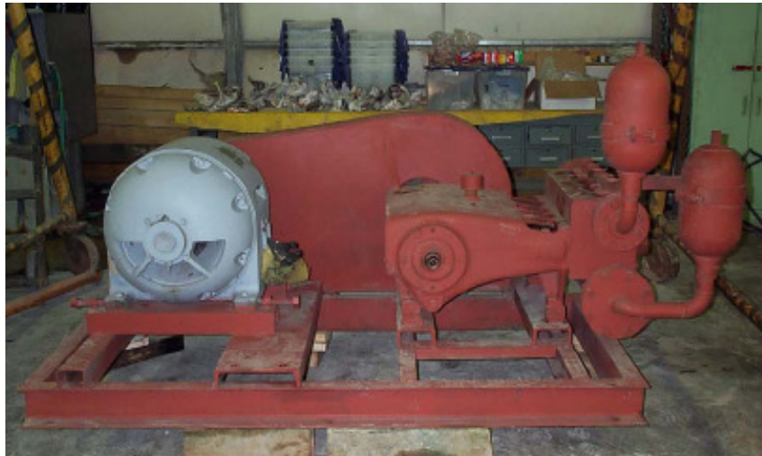
Figure 4.2 Wheatley Quintuplex high-pressure pump
