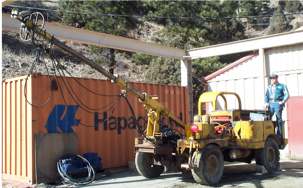
Figure 4.6. The CSM waterjet carrier vehicle
