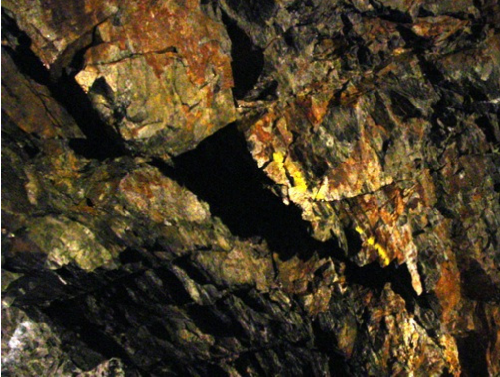
Figure 6.44 Void created by waterjet during Experiment #8
