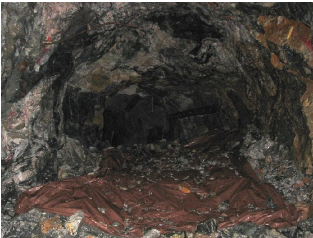
Figure 6.31 Material removed in Experiment #6 waterjet test
