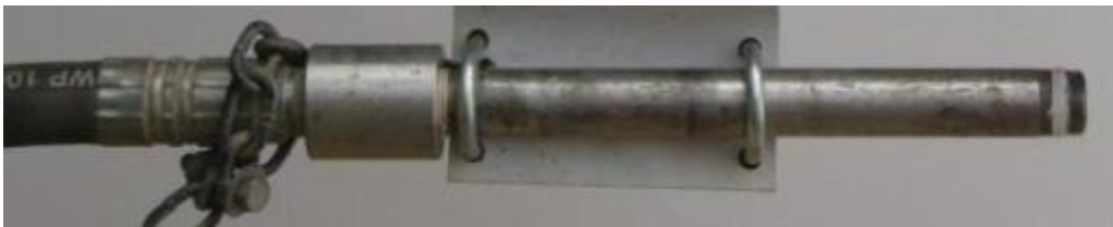
Figure 4.7. High pressure hose, female end fitting, and pipe.
