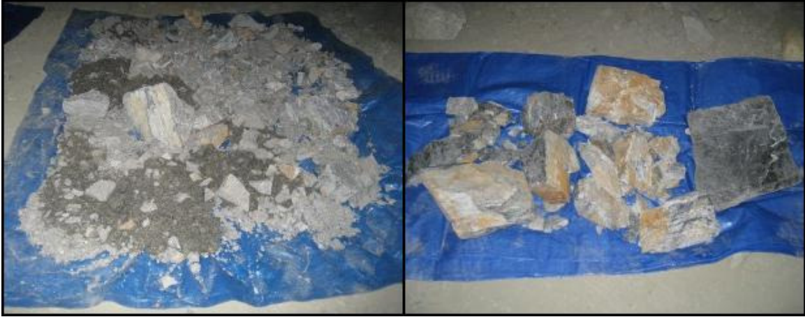
Figure 6.5 Waterjet and Manual scaling results
