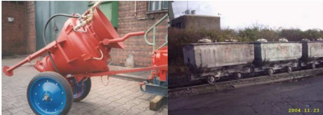
Figure 4.6 Small (left) and Large (right) Compressed Air Duster Units. Source: RAG Hauptstelle für das Grubenrettungswesen (RAG Mine Rescue Headquarters), Herne, Germany.
