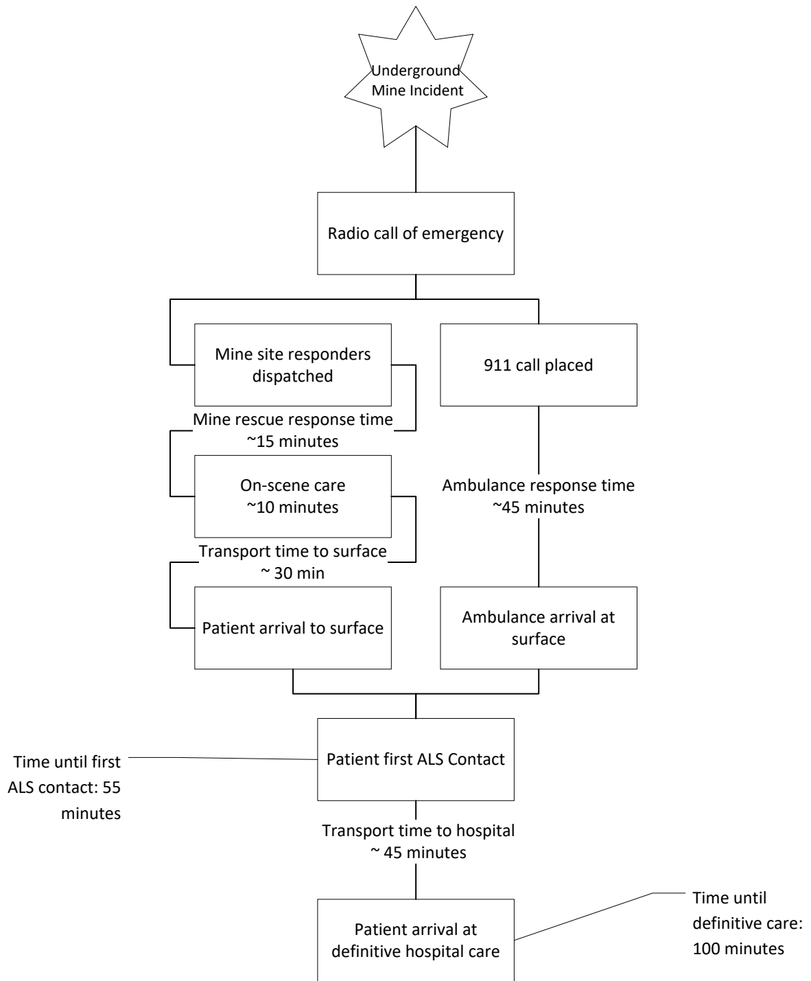
Figure 7.2: Conceptual timing for medical care for an underground mine accident. Times are assumed based on experience and data collected on transport times from mines to hospitals.
