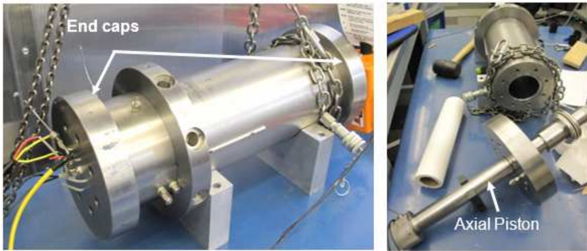
Figure 2.4: (Left) assembled triaxial testing cell displaying the end caps and (right) disassembled triaxial testing cell showing the internal axial piston (Padin 2016).
