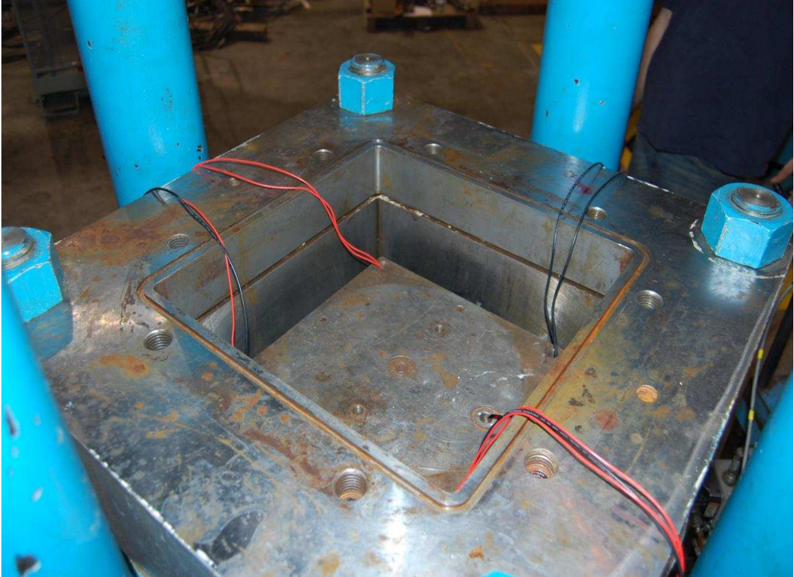
Figure 3.12 – Specimen in test frame ready for the vertical ram to be inserted and pressure applied. The wires running to the various acoustic sensors can be seen draped over the sides of the test frame.
