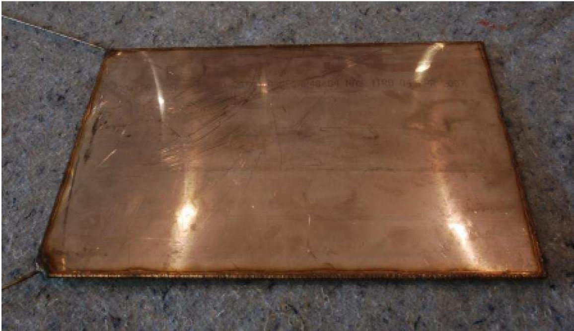
Figure 3.10 – High pressure flat jack shown on its side.
