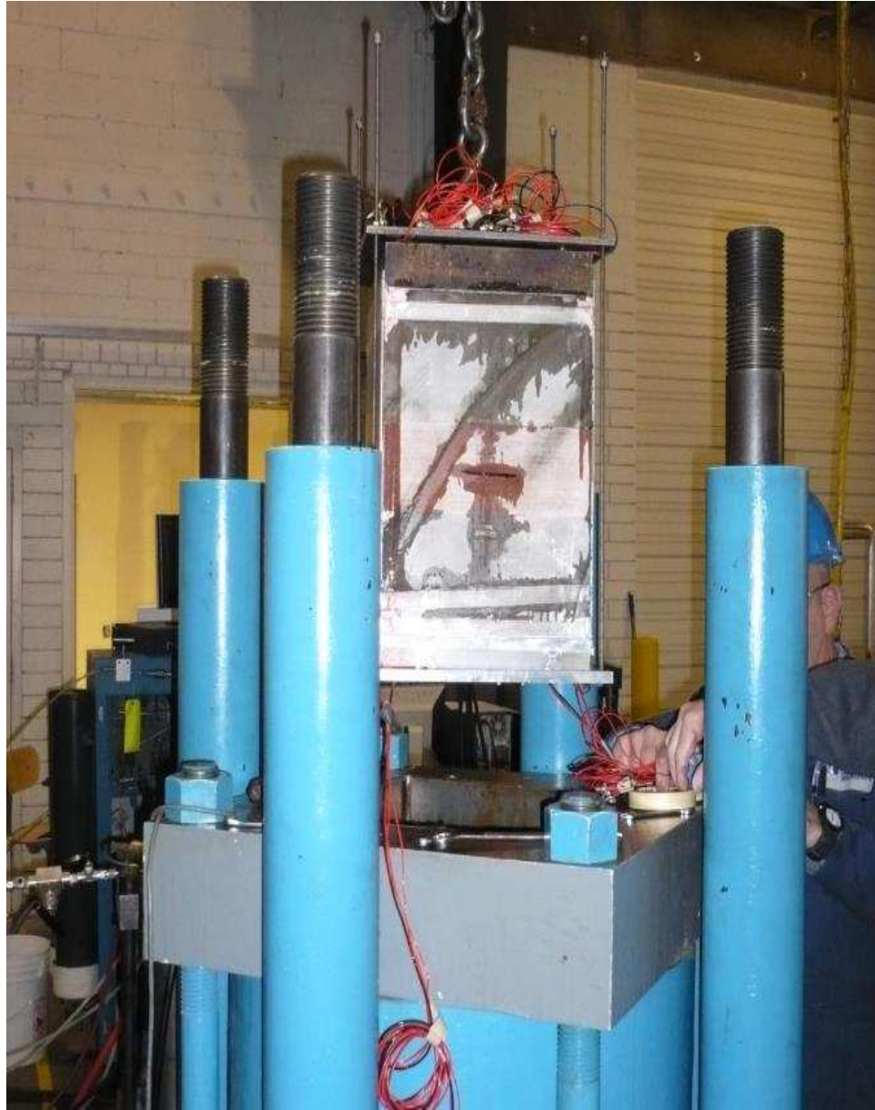
Figure 3.11 – Test block being lowered into the test frame.
