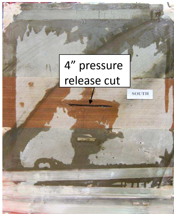
Figure 3.5 – Block after fracture showing pressure release cut on the outside of the block.
