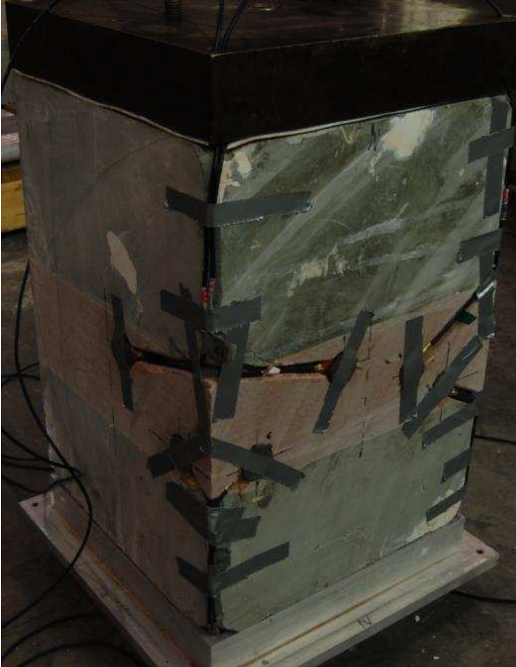
Figure 3.8 – Receivers and cables protected with duct tape and ½” of high density foam prior to being place in the tri-axial test frame.
