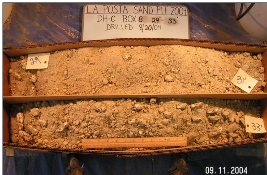
Figure 4.7: Four foot sample interval of DG obtained through sonic drilling.
