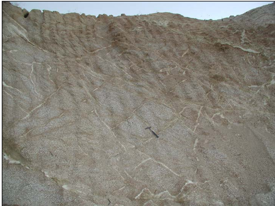
Figure 4.1: Clay seams along the southeastern wall of the Sand Pit, hammer for scale. Also visible are tooth marks made by ripping during the previous mining operation.
