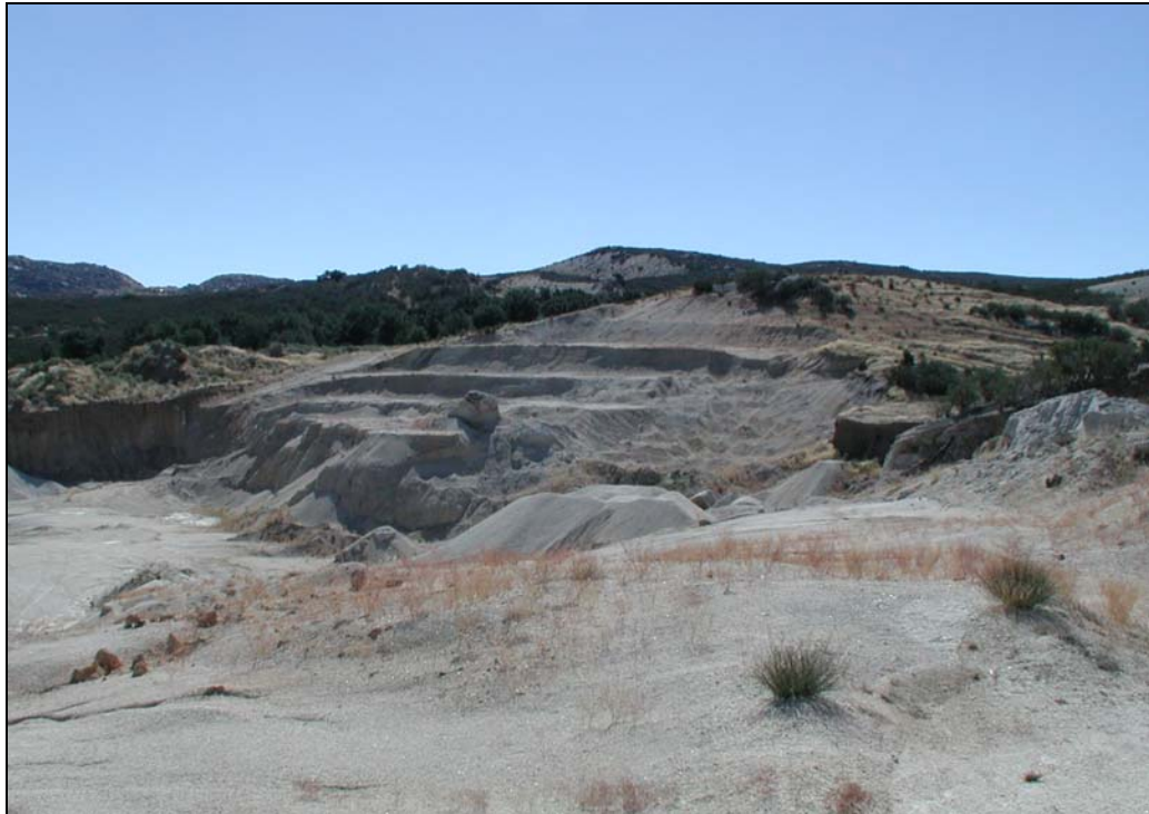
Figure 1.4: Benches on the south side of the inactive Sand Pit. All material previously excavated was “ripped” with a track-hoe. Note unweathered boulder protruding from the center of the ripped face.
