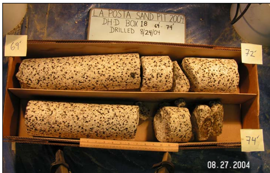
Figure 4.8: Sample of sonic drilling through competent rock.
