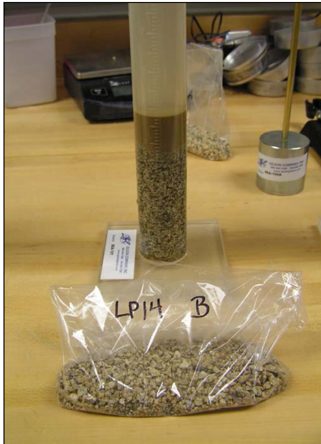
Figure 3.5: Sand equivalent test on surface sample LP14.
