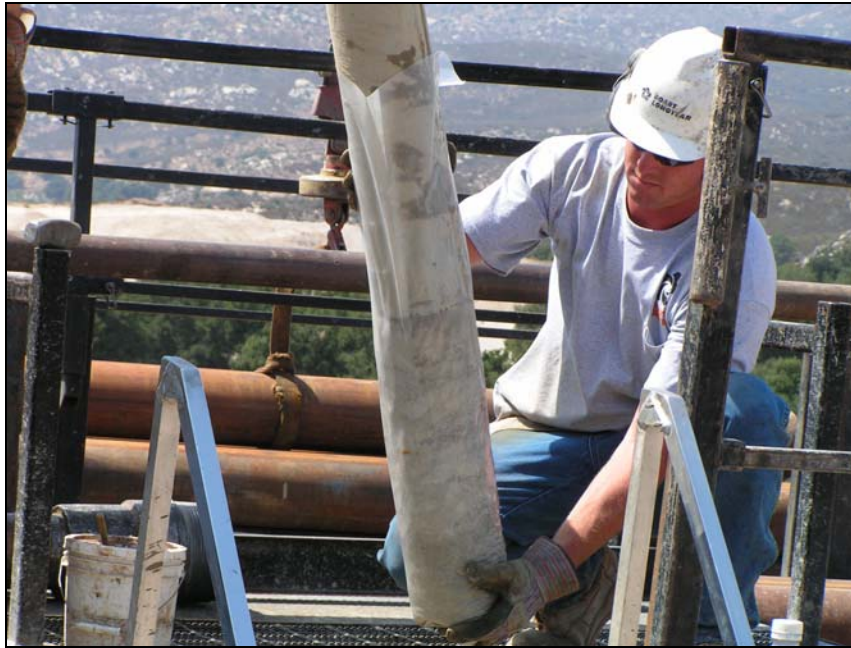
Figure 3.3: Sonic drilling sample being extruded from sampling tube.
