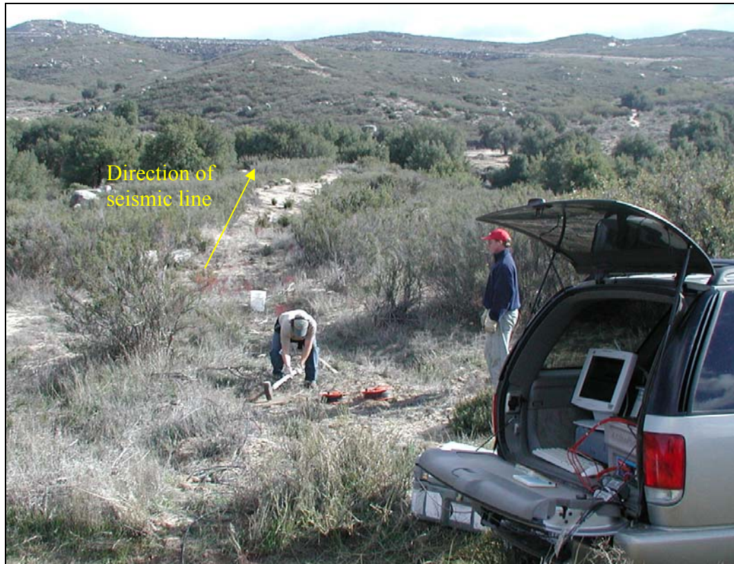
Figure 3.1: Sledge hammer impact on a steel plate was used as the seismic energy source for the geophysical surveys. Photograph shows LP-S5 location and computer used for data collection.
