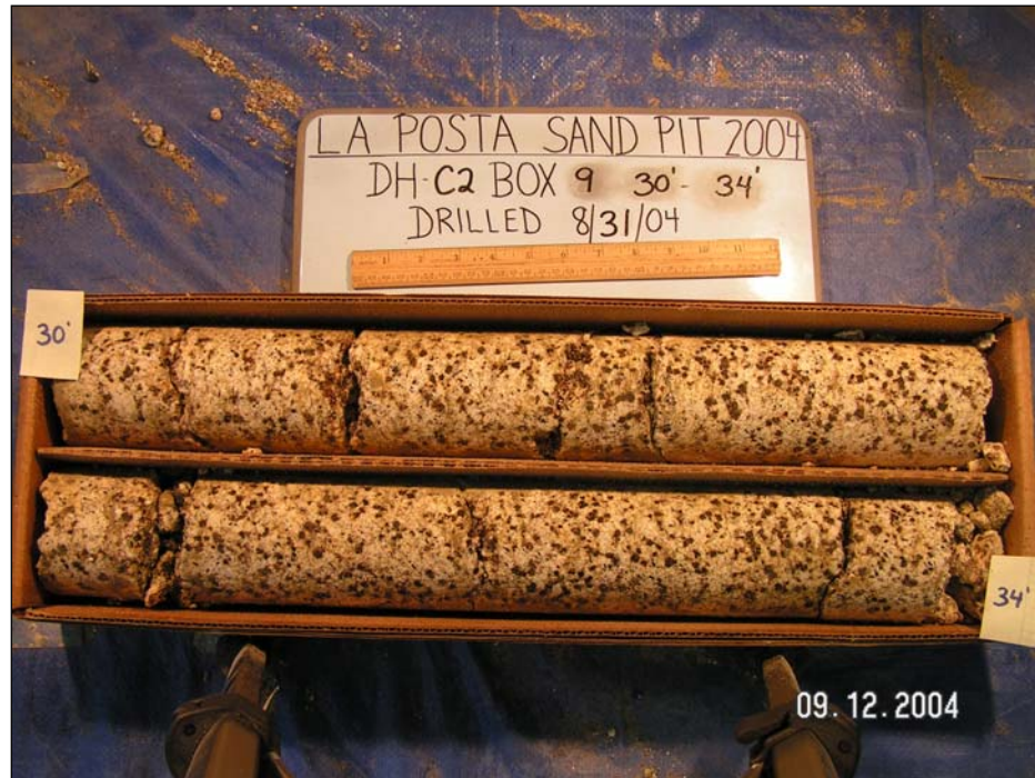
Figure 4.9: Four foot interval of DG drilled by wireline core; note this sample is collected from a twinned hole from approximately the same depth as Figure 4.7.
