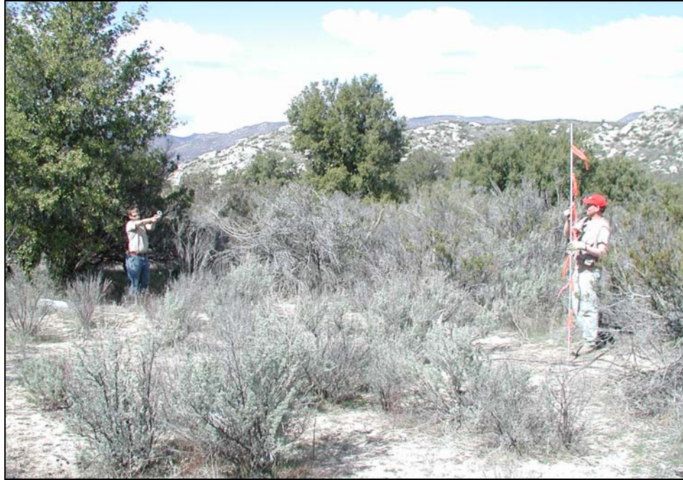
Figure 3.2: At LP-S4, a Brunton pocket transit (compass) and survey staff were used to measure elevation changes.
