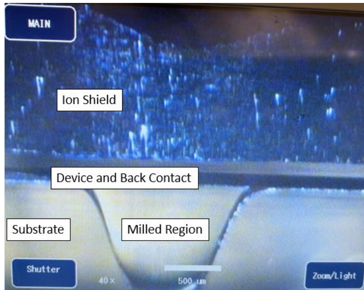
Figure 2.4 An extreme case of in situ Ion Mill results. The ion shield acts as a sacrificial layer to prevent damage to the sample. The milled region is a roughly gaussian distribution caused both by the sputtered ion trajectories as well as the sample rocking procedure which reduces mill curtaining effects.
