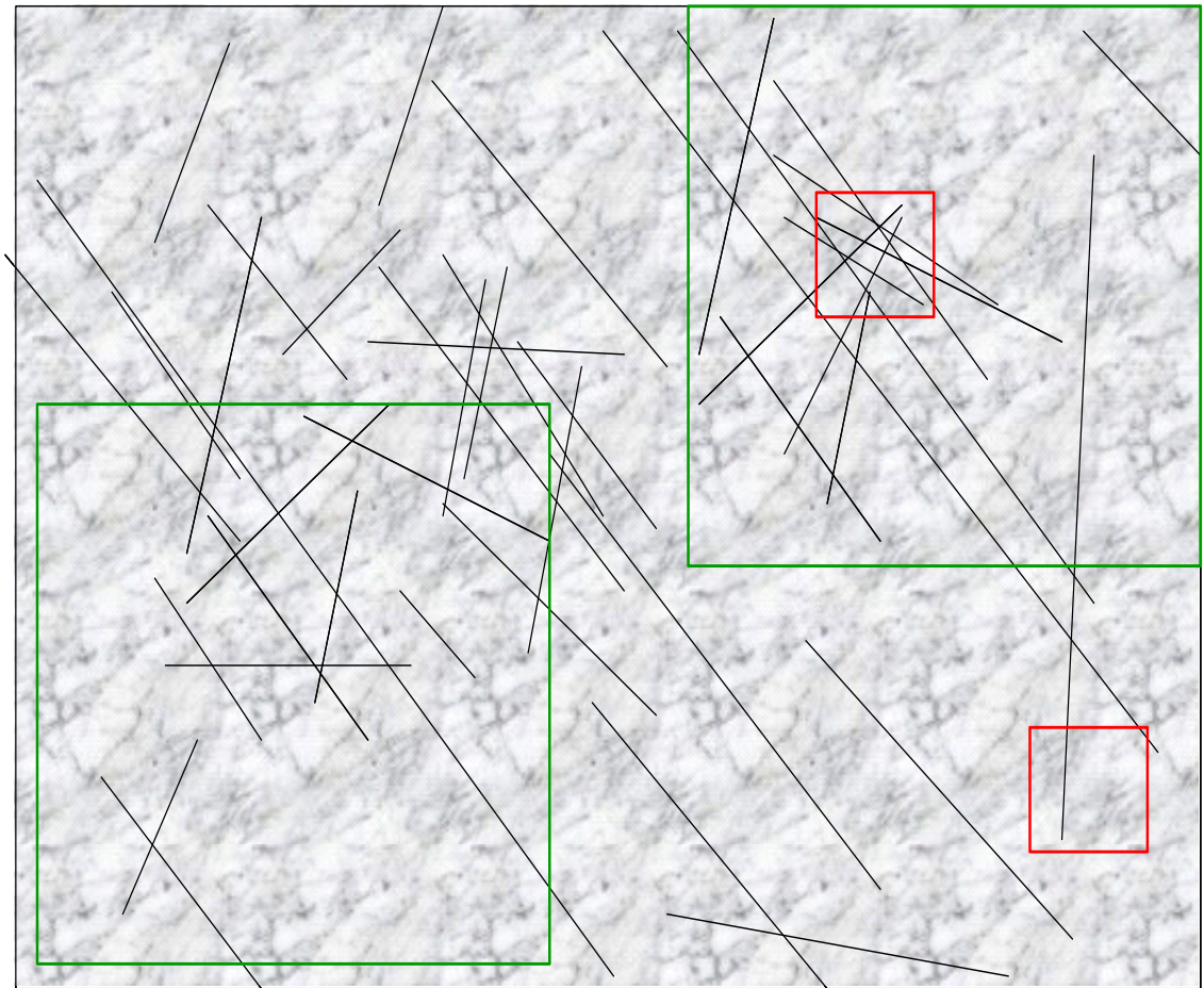
Figure 4.1 Two-dimensional representation of a fractured medium, squares represent sample areas.
