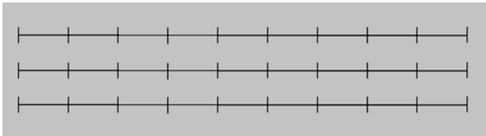
Figure 3.1: Non-Zipper Hydraulic Fracture Configuration.
