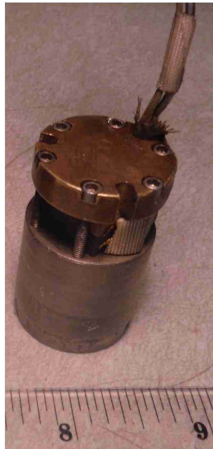
Figure 2.17: Lithium Niobate ( \text{LiNbO}_3 ) transducer. Diagram (left) and actual transducer (right)
