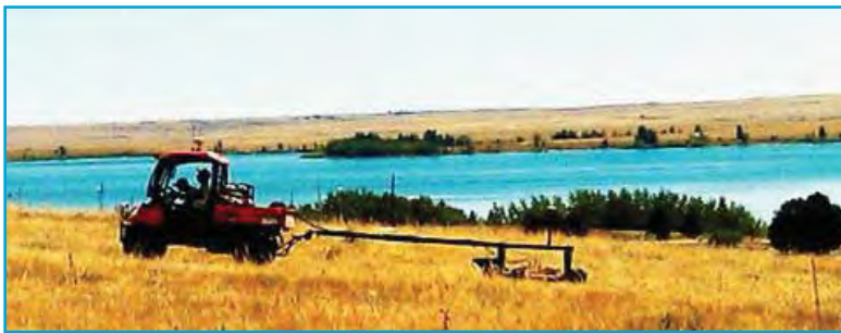
Kubota with towed-array of electromagnetic coils. Picture courtesy of Baraa Alrikaby, Sky Research
