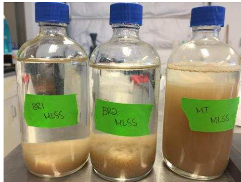
Figure 3.17. Sludge settling characteristics of BR1, BR2, and the MT over a 30-minute period. The poor settling of the MT sludge is the reason for not recycling sludge back into the BRs.
