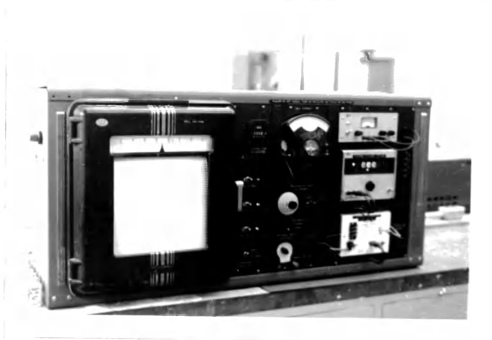
Figure 5 - View of the control panel for electrolysis
