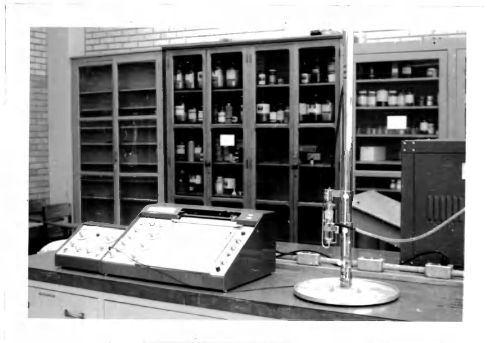
Figure 6 - View of the polarograph used for the determination of the electrocapillary curves
