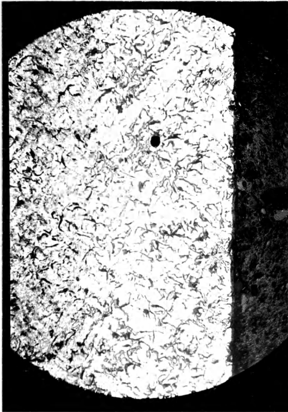
Figure 15--Microstructure of ferrite layer of sample 12R 100X (picral etch.)
