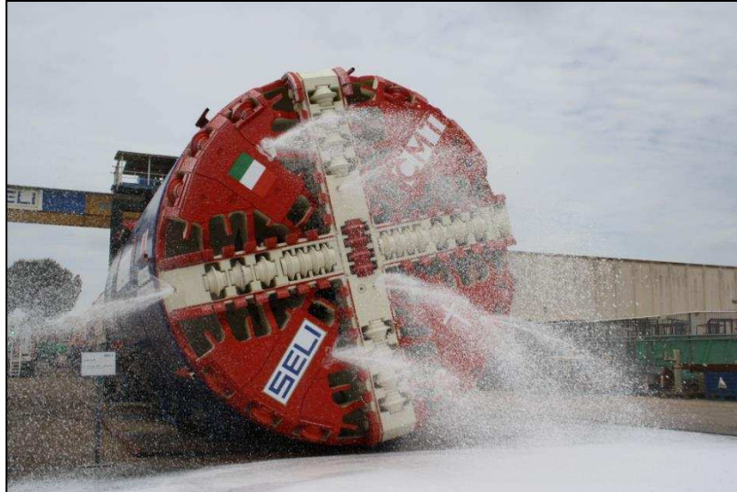
Figure 1.2 Aqueous foam injected through the foam port from the cutter head on a TBM
