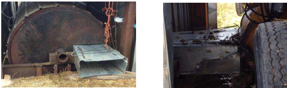
Figure 1.6: Left - Transfer housing is placed into the rolling drum. Right - Trailer is connected to the housing and able to transfer material.
