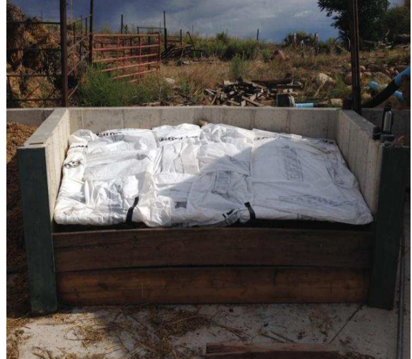
Figure 1.12: From left to right, top to bottom: Bobcat moves material into the aeration bin from the drum exit. Grass/hay is spread over the composting material in the bin. Wooden slats placed in front of the pile retain the material. A cover is placed over the top of the pile.
