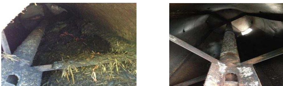
Figure 1.7: Interior of the rolling drum with and without any compost material inside.
