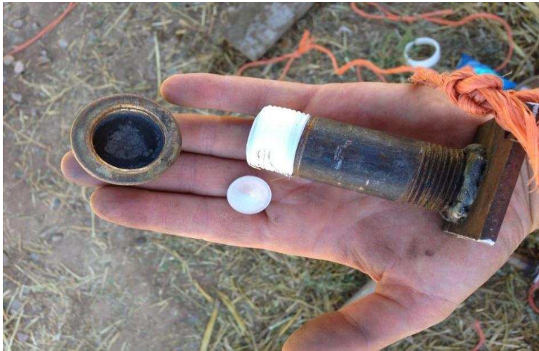
Figure 1.8: Temperature Vessel for Smart Buttons, and a Smart Button temperature sensor.
