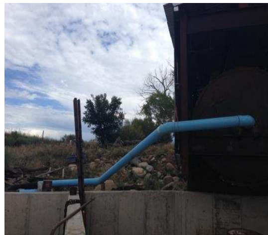
Figure 1.11: Left: Aeration tubes in the bins which must be seated to provide aeration path. Right: Drum ventilation and fan supplying moist air and gases to the aeration tubes.
