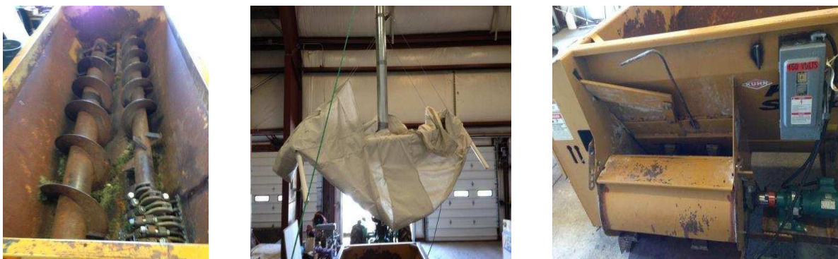
Figure 1.5: From left to right: grinding trailer, ventilation hood suspended by rope above the grinder, and the 1/8 hp electric motor attached to the grinder.
