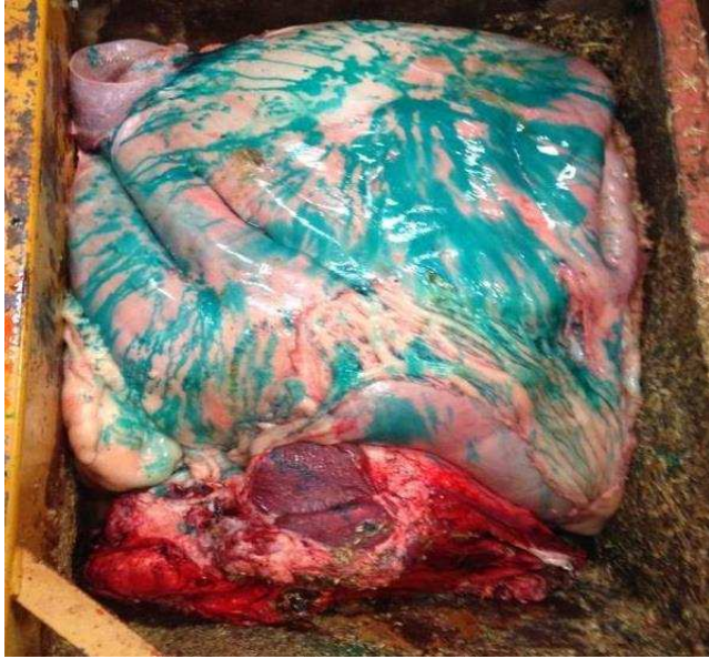
Figure 1.3: Denatured material from the kill floor, purposely dyed blue, in the grinding hopper.
