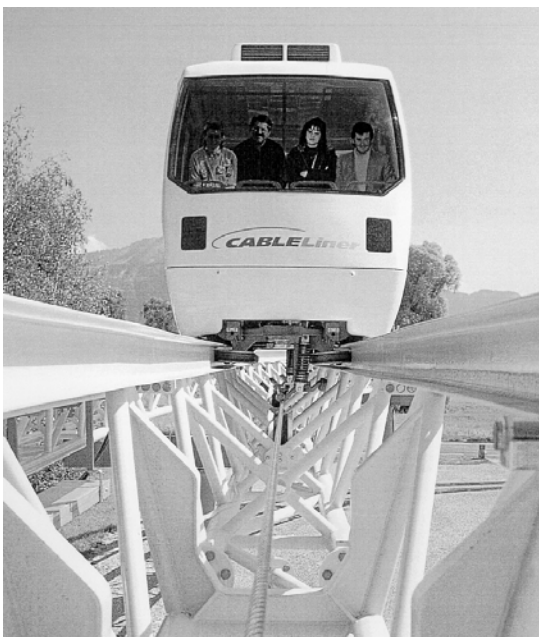
Figure 2b: Central rope, DCC /2/
