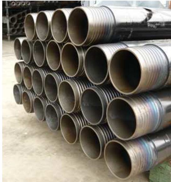
Figure 1.3: Traditional steel production casings used in the petroleum industry. Image used from ( https://www.collidrill.it/our-production/ accessed 4/25/19)
