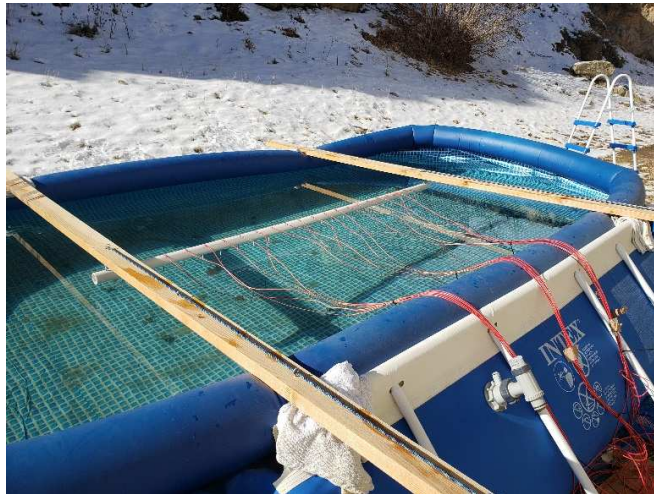
Figure 3.1: Photograph of the lab-scale pool experiment. A 2-inch-thick PVC pipe is suspended between two large pieces of lumber by rope allowing the PVC pipe to be lowered down to the water. Nineteen galvanized steel electrodes are driven through the pipe at 0.10 m intervals for a total array length of 1.8 m. The electrodes are attached to insulated 12 AWG wire running out of the pool and connected via banana plugs to the AGI USA SuperSting R8 DC resistivity instrument.
