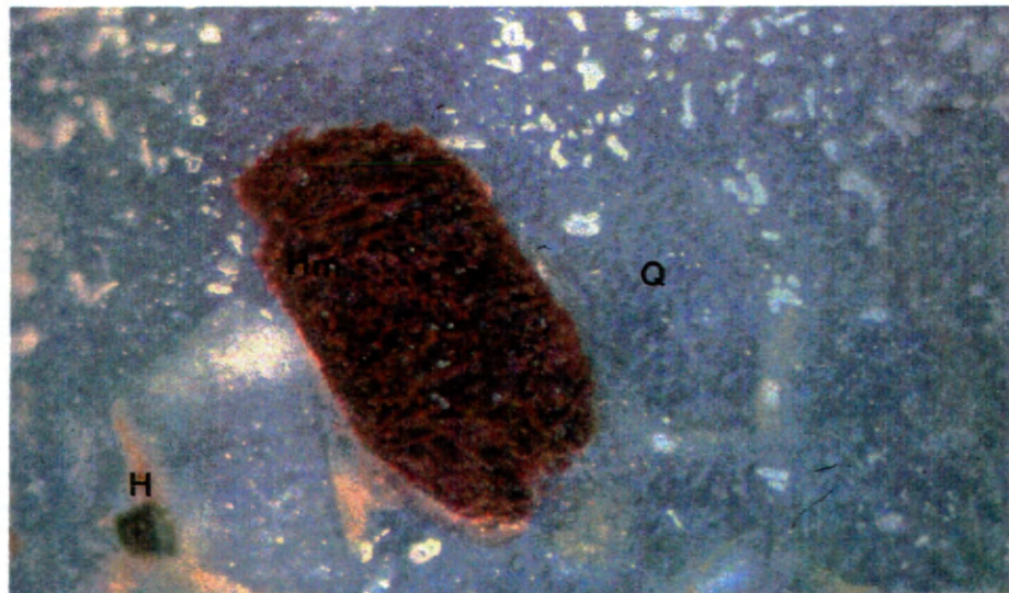
Figure 13: Photomicrograph in oblique reflected light of hematized detrital magnetite grain (Hm), hematite within quartz overgrowth (H) and detrital quartz grains (Q). Field of view = 0.2 mm wide.
