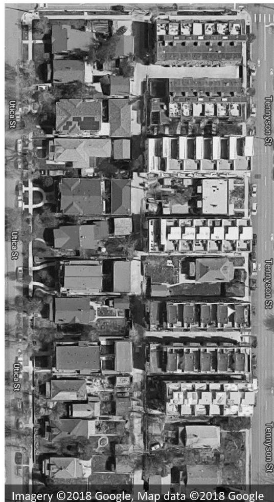
Figure 2.1 Example aerial image of infill development occurring along Tennyson Street in the Berkeley neighborhood of Denver, CO. The left side of the image shows single family homes with lawns, while the right side illustrates the increase in impervious area of redeveloped multi-family units. (Source: Google Maps)
